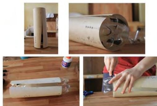
Figure 5 – Definitive template for PET bottle cutting (Author, 2013).
