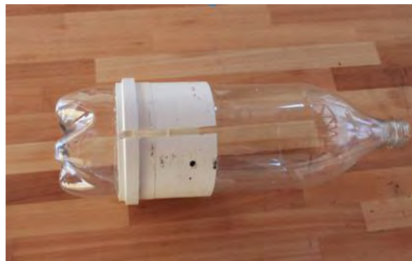
Figure 4 – First template for PET bottle cutting (Author, 2013).
