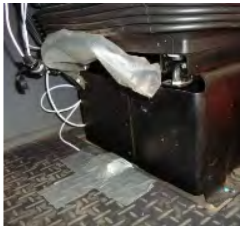
Figure 2. Fixing the accelerometer in the region of the floor.
