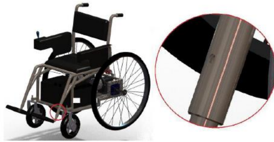
Figure 5. Guide tube detail. That tube allows the foot set up.
