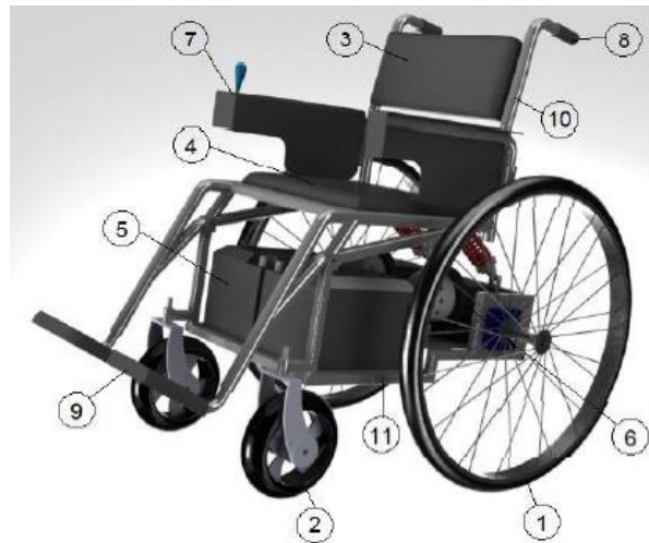
Figure 2. Wheelchair parts; 1- Rear wheel; 2- Front wheel; 3- Back suport; 4- Bottom; 5- Batteries; 6- Transmission system; 7- Joystick; 8- Paw; 9- Foot support; 10- Wheelchair structure; 11- Batteries and engine structure.
