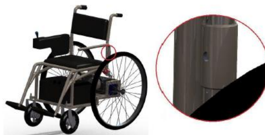
Figure 4. Guide tube detail. That tube allows the arm set up.
