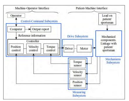
Figure 2. Block diagram of the ID.
