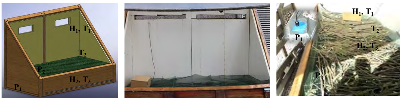
Figure 1. Solar kiln: P_1 – external pyranometer; P_2 – internal pyranometer; T_1 – thermocouple, upper part; T_2 – thermocouple, middle; T_3 – thermocouple, lower part; H_1 – air relative humidity sensor, upper part; H_2 – air relative humidity sensor, lower part.
