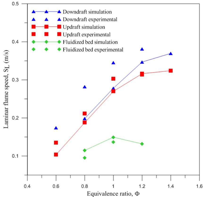
Figure 1. Simulation and experimental (Monteiro *et al.*, 2009) comparison of laminar flame speed for three wood gas compositions at atmospheric pressure and unburned gas temperature of 293 K.
