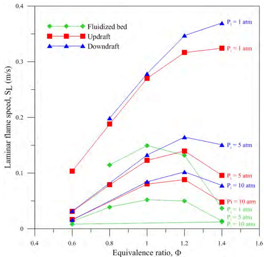
Figure 3. Unburned gas initial pressure influence on laminar flame speed of the three wood gas mixtures,  $T_i = 293$  K.
