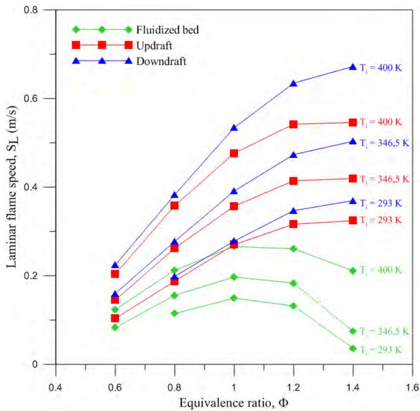
Figure 2. Unburned gas initial temperature influence on the laminar flame speed  $S_L$  of the three wood gas mixtures at atmospheric pressure.
