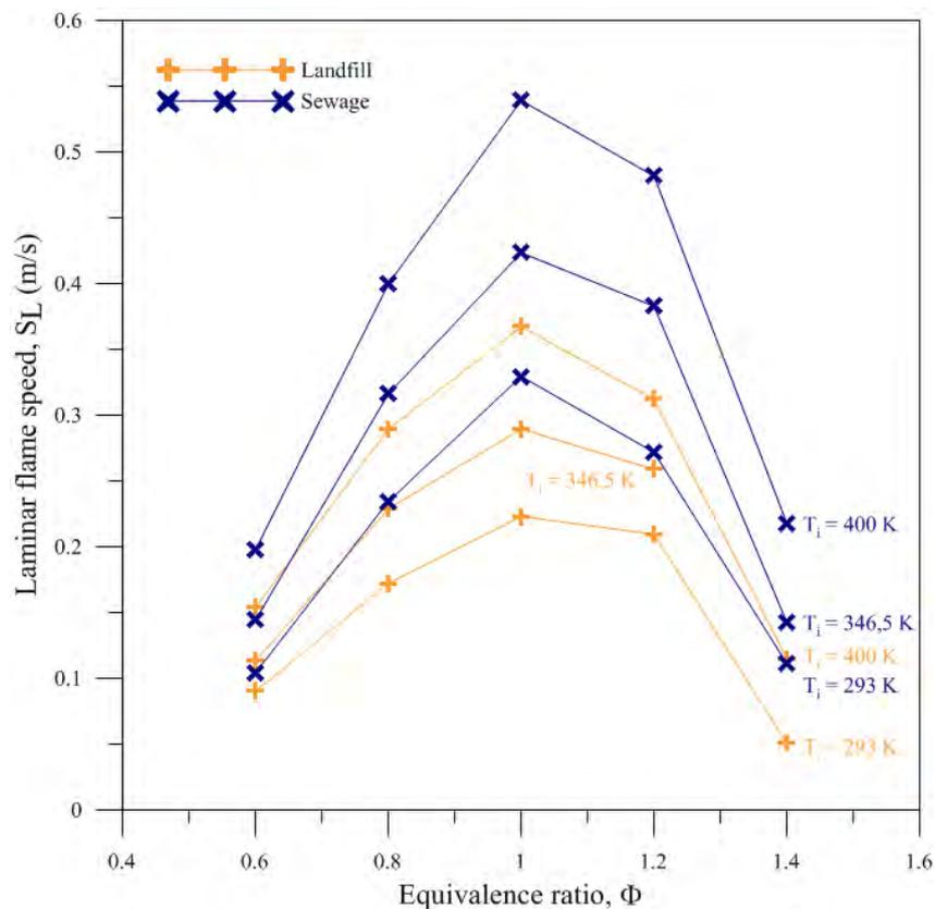
Figure 4. Unburned gas initial temperature influence on the laminar flame speed
