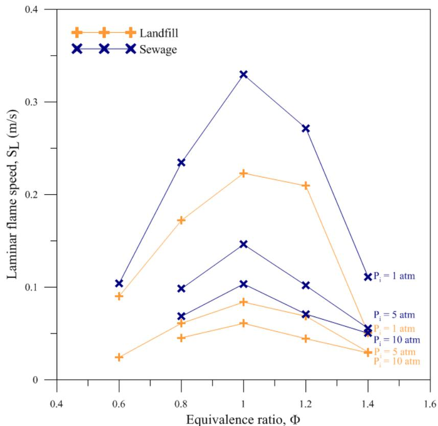
Figure 5. Unburned gas initial pressure influence on laminar flame speed of landfill and sewage gases at  $T_i = 293$  K.
