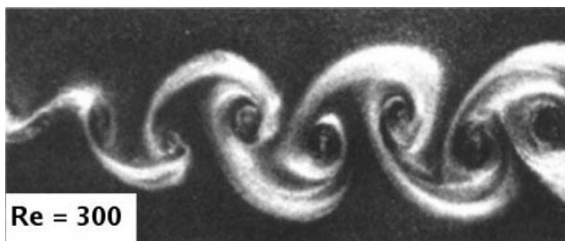
Figure 1. Von Karman vortex formation at Re = 300
