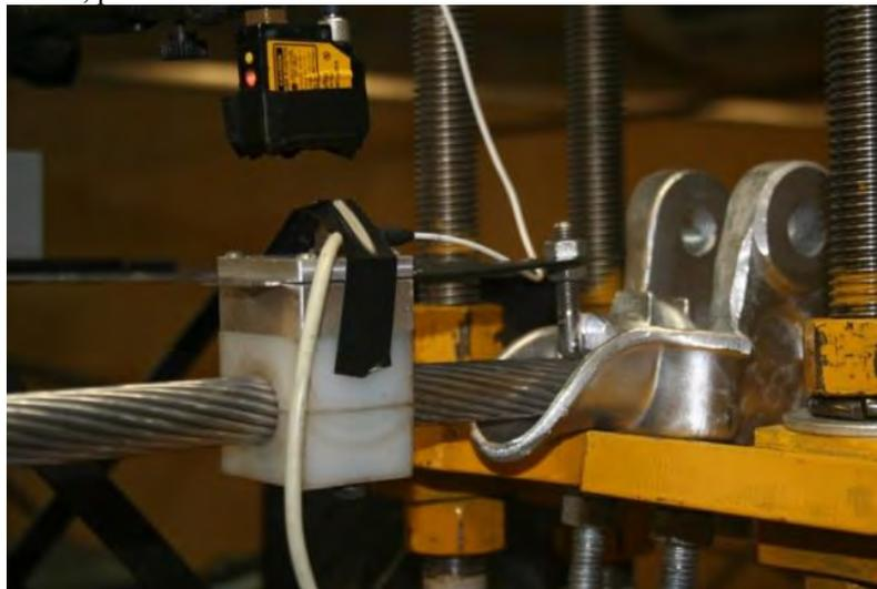
Figure 2.13 - Sensor Measuring System Installed in reverse.
