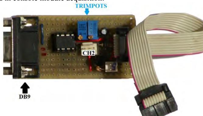
Figure 2.7: Operational Amplifier Board.
