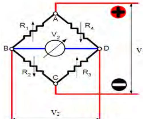
Figure 2.4: Arrangement of the blade strain gauges on Wheatstone bridge circuit.
