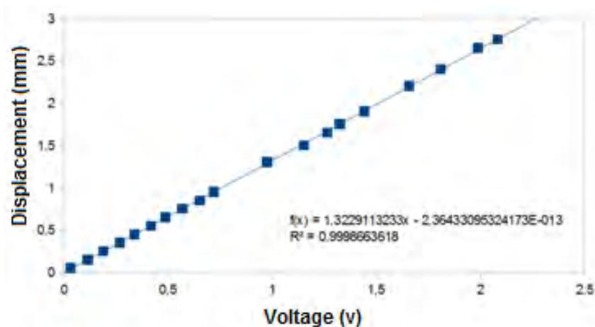
Figure 4.1 - Calibration curve for gain 600.
