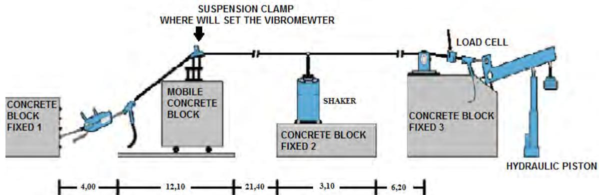
Figure 2.11 - Schematic drawing of the assembly test bench (modified - Fadel, 2010)
