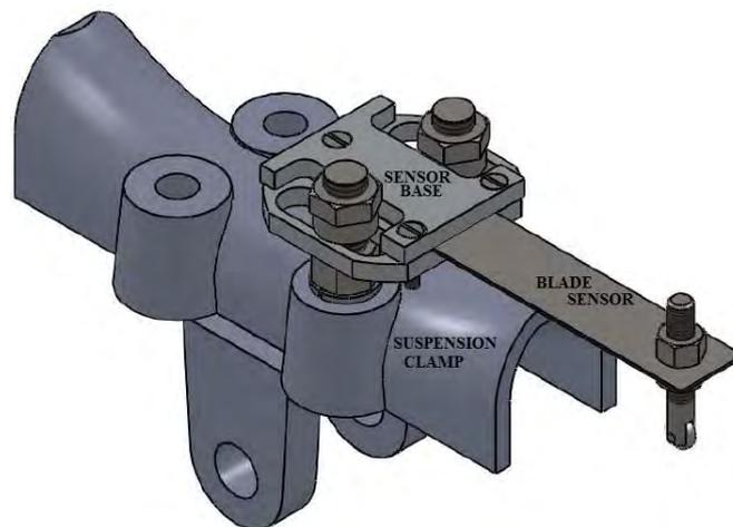
Figure 2.1 - Format and method of attachment of the base vibrometer for the direct measurement of the cable suspension clamp.
