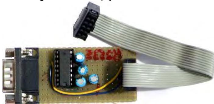
Figure 2.8 - RS232 communication board.
