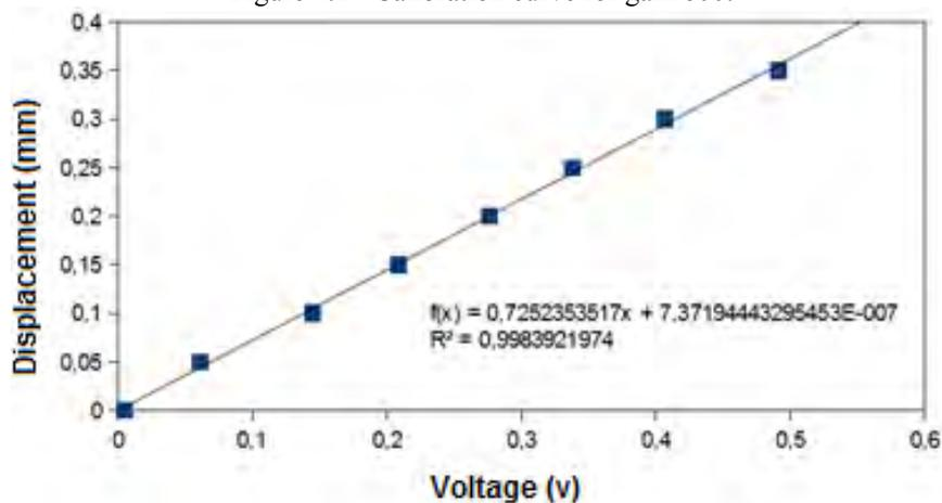
Figure 4.2 - Calibration curve for gain 1000.
