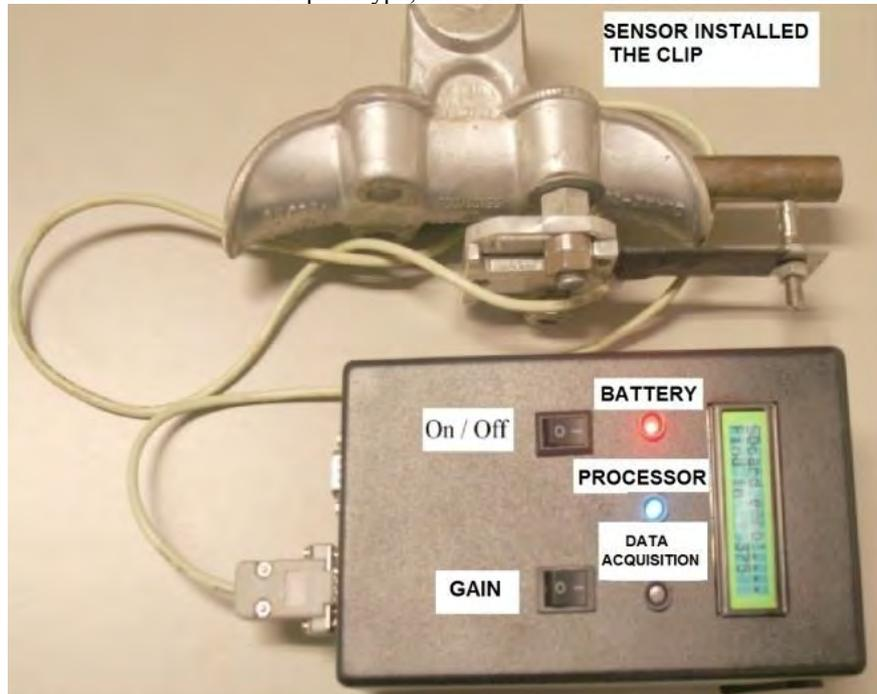
Figure 2.9 - Current vibrometer prototype, external view.
