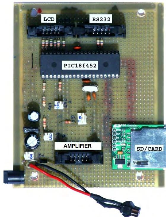
Figure 2.6 Construction of physical main board of the vibrometer
