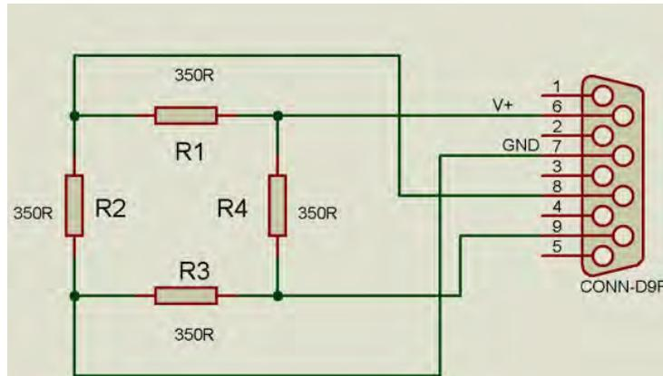
Figure 2.5 - Load cell circuit.
