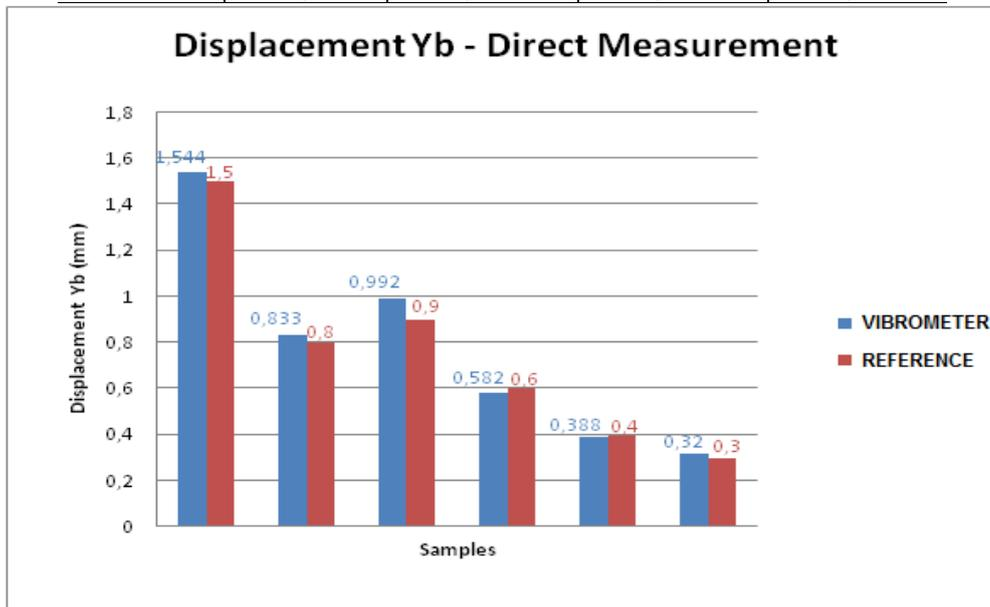
Figure 4.3 - Graphical representation of comparative Yb offset values between Vibrometer in direct measurement setting and laboratory reference.
