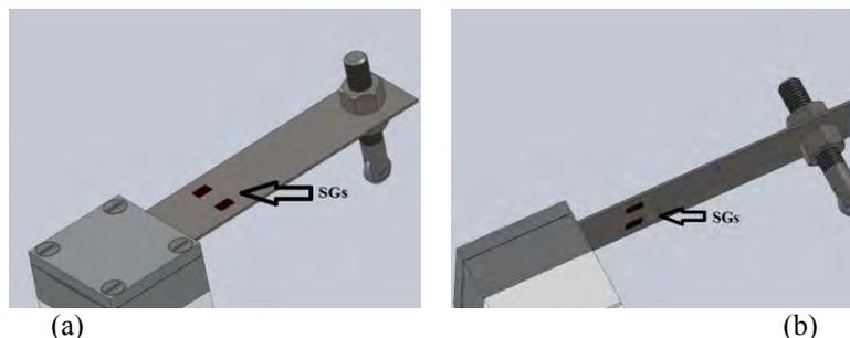
Figure 2.3 - Positioning of SGs in the faces of the blade. (a) Top view. (b) Lower panel.
