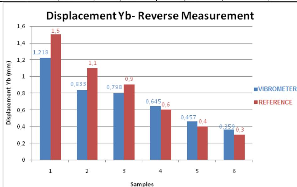
Figure 4.4 - Graphical representation of comparative offset values Yb between Vibrometer in reverse measurement setup and the laboratory reference.
