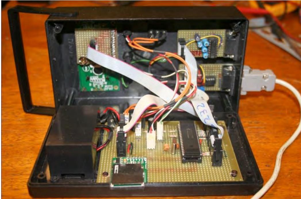
Figure 2.10 - Current vibrometer prototype, inside view.
