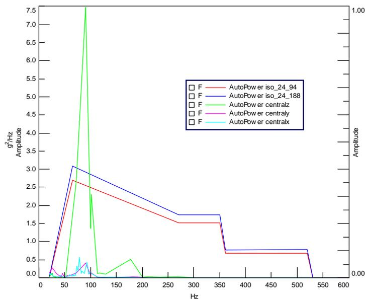
Figure 7. Comparison between accelerated PSD's of Sine-on-random tests specified by ISO and application accelerated PSD.
