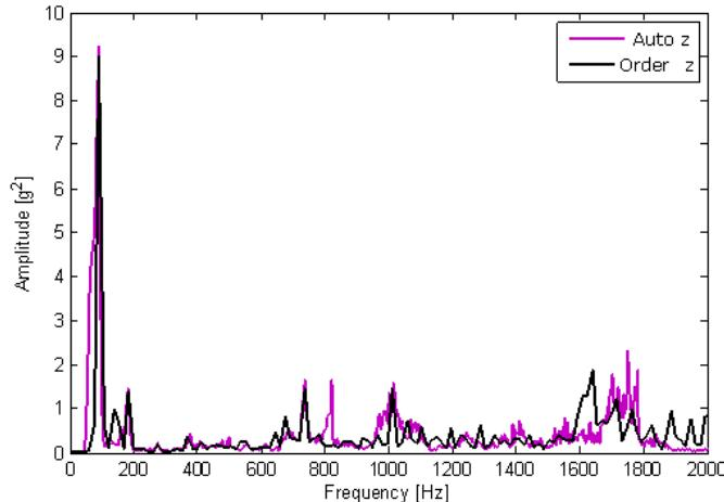
Figure 6. Actuator vibration spectrum and engine order at vertical direction.
