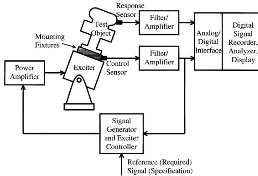
Figure 2. Electrodynamics driver used for vibration test (Silva, 2000).
