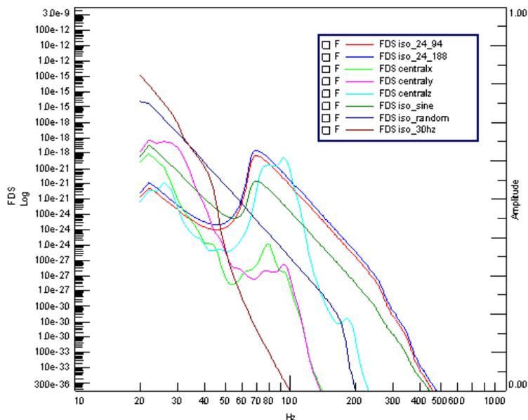
Figure 9. Fatigue Damage Spectrum Comparison.
