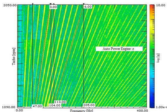
Figure 4. Vibration Waterfall plot (6 cylinders engine)
