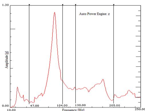
Figure 5. Vibration Spectrum Peak Hold (6 cylinders engine)
