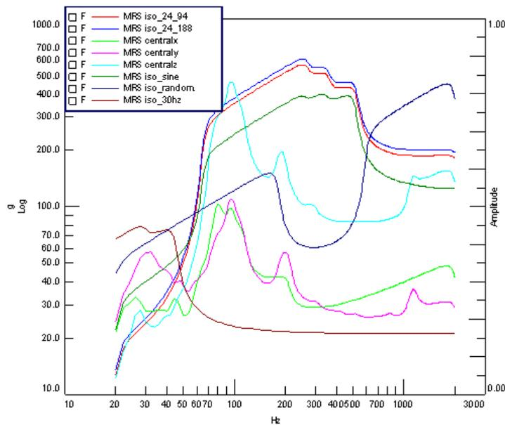
Figure 8. Maximum Response Spectrum Comparison.
