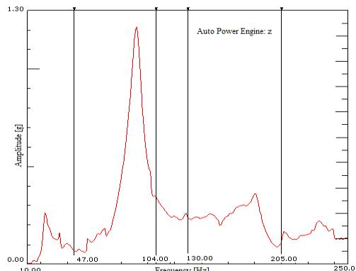
Figure 5. Vibration Spectrum Peak Hold (6 cylinders engine)
