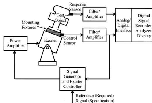
Figure 2. Electrodynamic driver used for vibration test (Silva, 2000).
