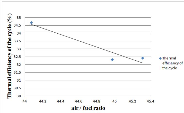
Figure 9 - Thermal efficiency of the cycle in relation air/fuel ratio
