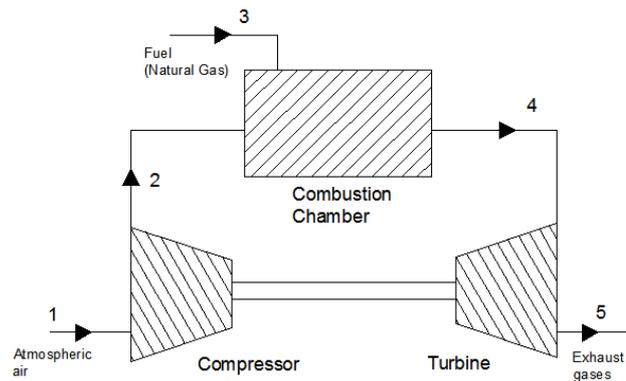
Figure 1 - Schematic representation of the gas turbine
