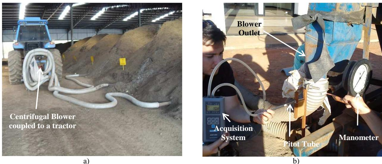
Figure 8. Aeration in organic compost piles a) Blower coupled to a tractor and organic compost piles; b) Experiment to determine the mechanical characteristics of the blower.
