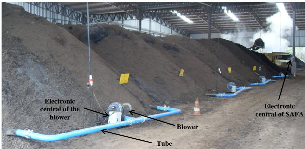
Figure 10. SAFA installed in the compost shed.
