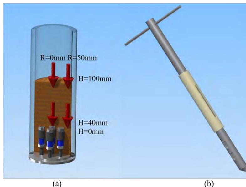
Figure 6. (a) Schematic of samples regions of the bed (b) Design sampling probe.
