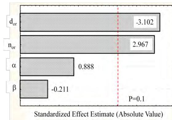
Figure 8. Pareto Diagram for the effect of for mixture mass density.
