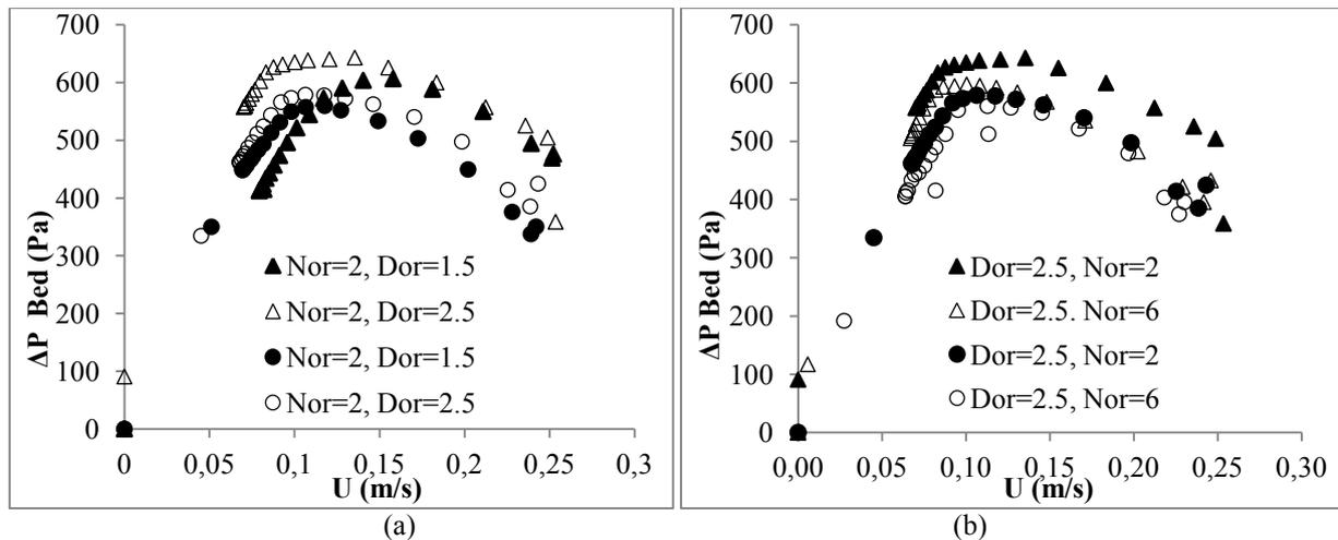
Figure 9. Hydrodynamics curves modifications for the two statistical relevant variables: (a)  $d_{or}$  (b)  $n_{or}$ .
