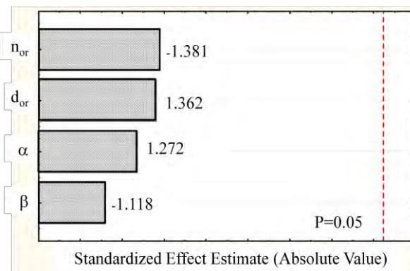
Figure 7. Pareto Diagram for the effect of Minimum fluidizing velocity.
