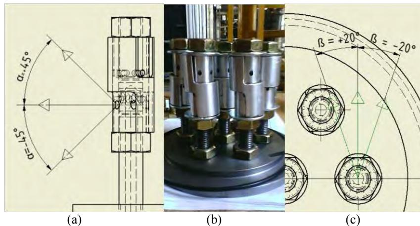
Figure 3. (a) Schematic of alignment angular positioning of the towers; (b) Picture of distributor design used in this paper and (c) Schematic of alignment angle of the gas jet in the vertical direction of the tower.
