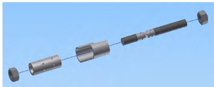
Figure 2. Exploded view of one tower of the tuyere distributor designed
