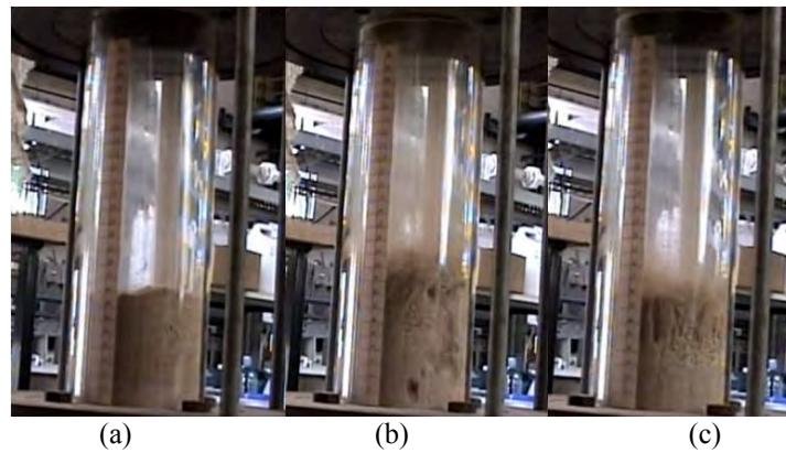
Figure 5. Different behaviors found in the tests: (a) Fixed Bed; (b) Bubble bed and (c) occurrence of preferential channels
