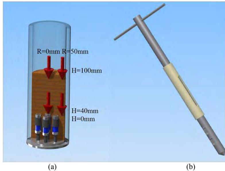
Figure 6. (a) Schematic of samples regions of the bed (b) Design sampling probe.
