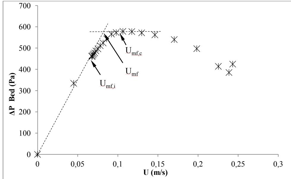
Figure 4. Methodology used to determine the minimum fluidizing velocities ( $U_{mf,i}$ ,  $U_{mf}$  and  $U_{mf,c}$ ).
