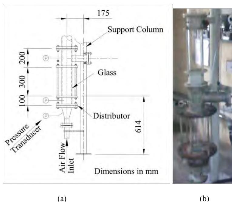
Figure 1. (a) Schematic diagram of the fluidized bed column (b) Picture of the main column.
