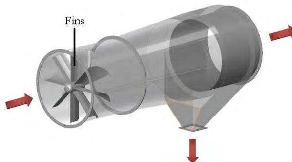
Figure 1. Pre-collector of particulates.
