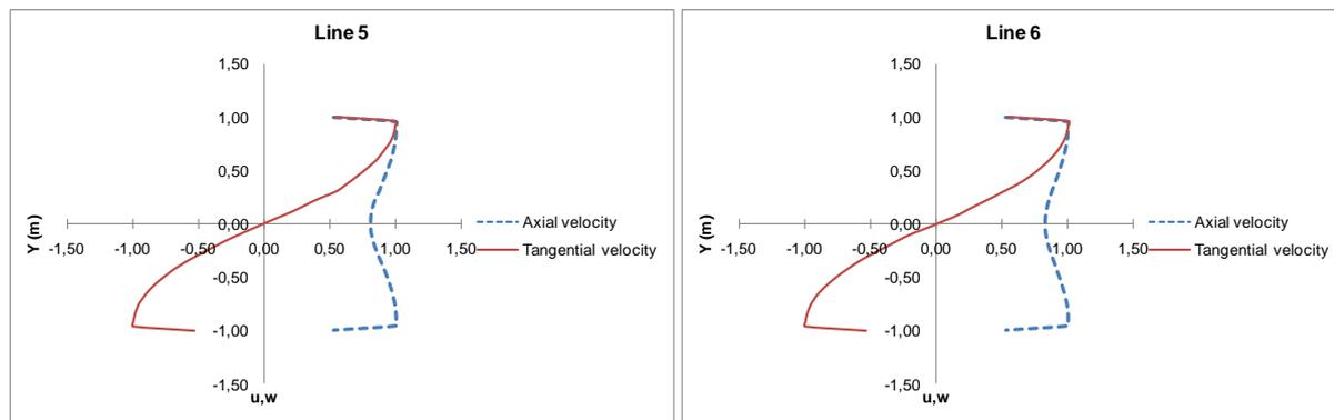
Figure 8. Profile of tangential and axial dimensionless velocities in the lines.
