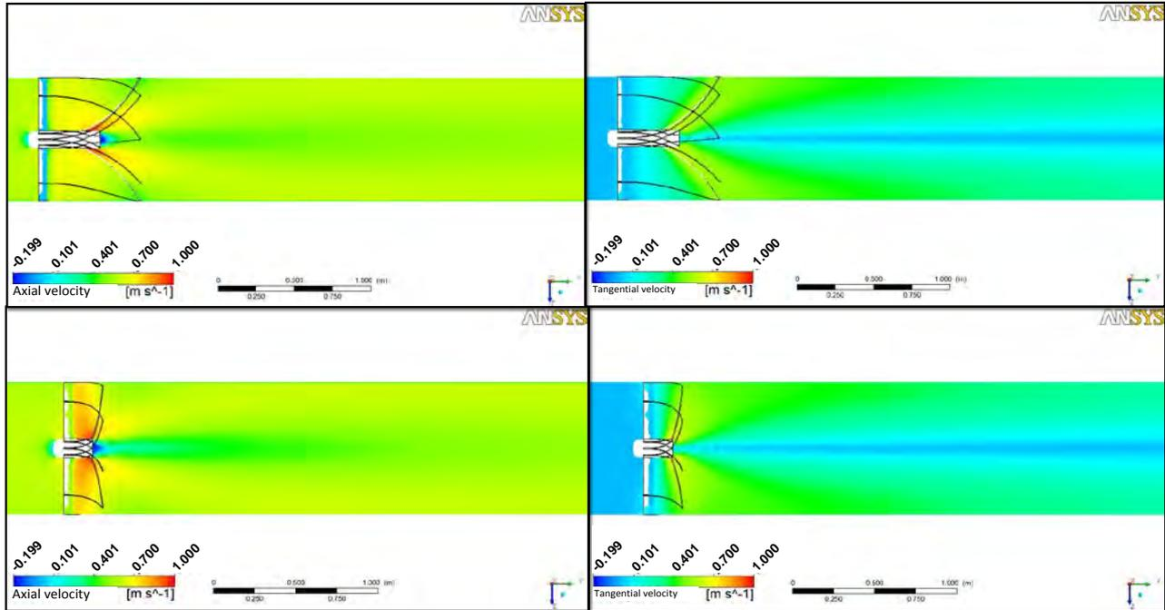
Figure 7. Axial and tangential dimensionless velocities of the combinations number 3 and 10 of Tab. 2.
