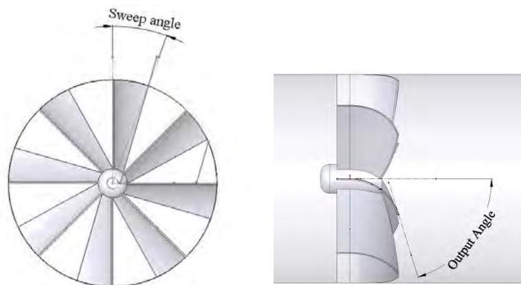
Figure 3. Details that show sweep angle and output angle.
