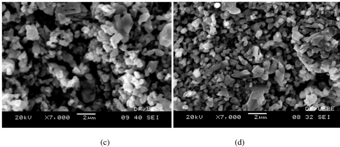
Figure 4 SEM micrographs of AZY ceramics: (a – 5wt% ZrO<sub>2</sub>, b – 10wt% ZrO<sub>2</sub>, c – 15wt% ZrO<sub>2</sub>, d – 20wt% ZrO<sub>2</sub>, all with 2wt% Y<sub>2</sub>O<sub>3</sub>)
