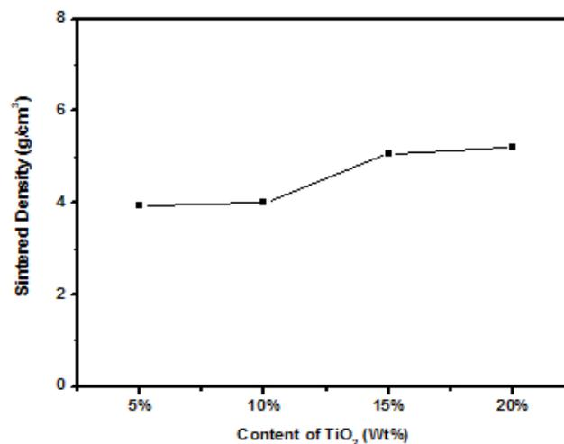
Figure 2 Sintered density of AZY ceramics
