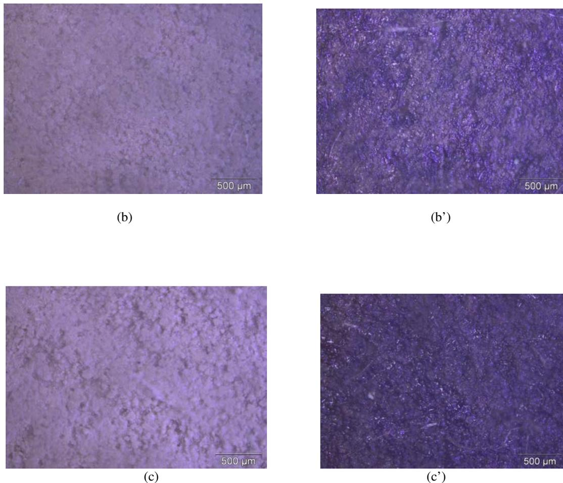
Figure 5. Optical micrographs of AZY ceramics in before and after submersion in crude petroleum. (a) and (a') Before submersion in crude petroleum, (b and b') after 60 days submersion in crude petroleum extracted from earthen petroleum wells, respectively and (c and c') after 60 days submersion in crude petroleum extracted from offshore petroleum wells respectively.
