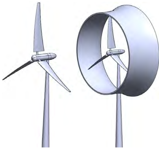
Figure 3. Wind turbine model without and with diffuser.
