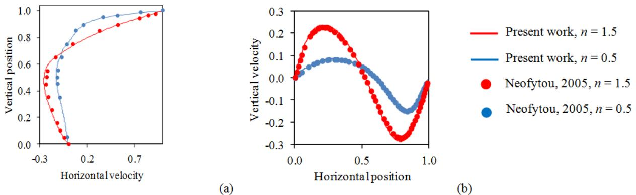
Figure 2: Results of present work and Neofytou (2005) for the lid-driven cavity. (a) Horizontal velocity versus vertical position and (b) vertical velocity versus horizontal position.
