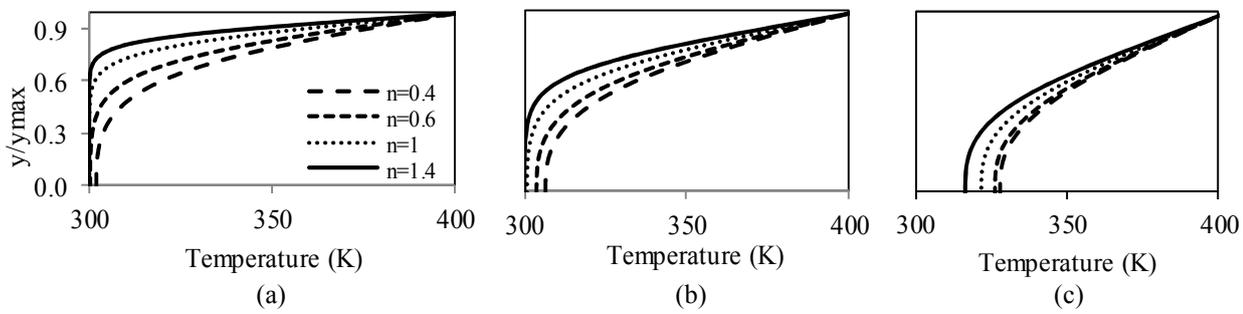
Figure 10. Temperature profile between the channel and cylinder wall,  $Pr = 50$ . (a)  $\beta = 0.25$ , (b)  $\beta = 0.5$  and (c)  $\beta = 0.75$ .
