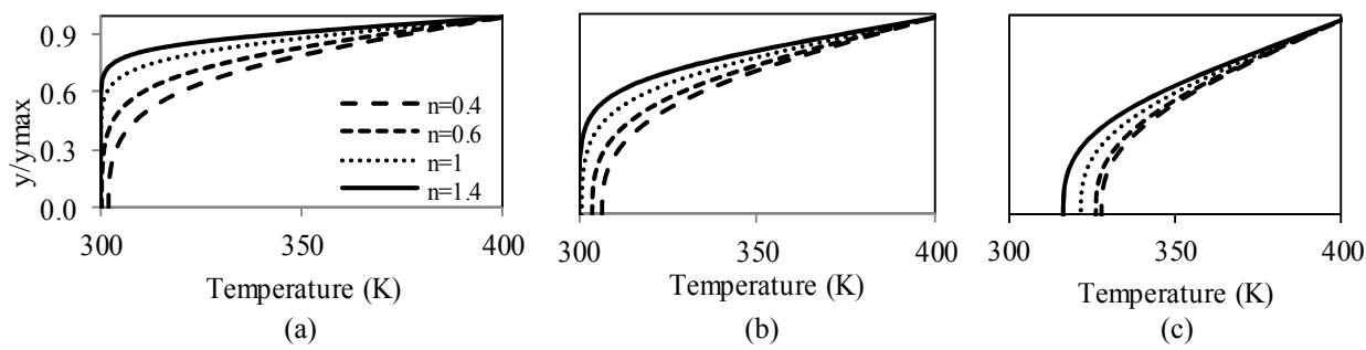
Figure 10. Temperature profile between the channel and cylinder wall,  $\text{Pr} = 50$ . (a)  $\beta = 0.25$ , (b)  $\beta = 0.5$  and (c)  $\beta = 0.75$ .
