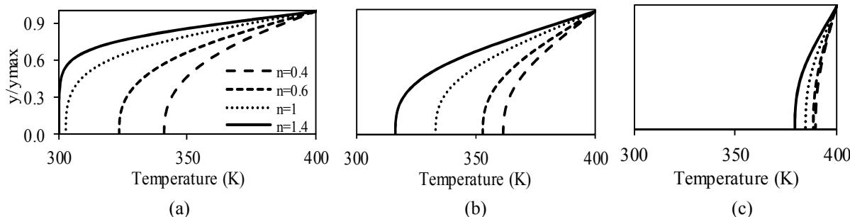
Figure 9. Temperature profile between the channel and cylinder wall,  $\text{Pr} = 10$ . (a)  $\beta = 0.25$ , (b)  $\beta = 0.5$  and (c)  $\beta = 0.75$ .
