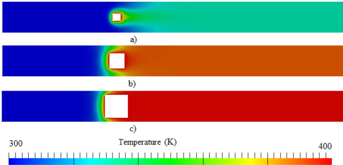
Figure 7. Temperature field for  $n = 0.4$ ,  $\text{Pr} = 10$ .
