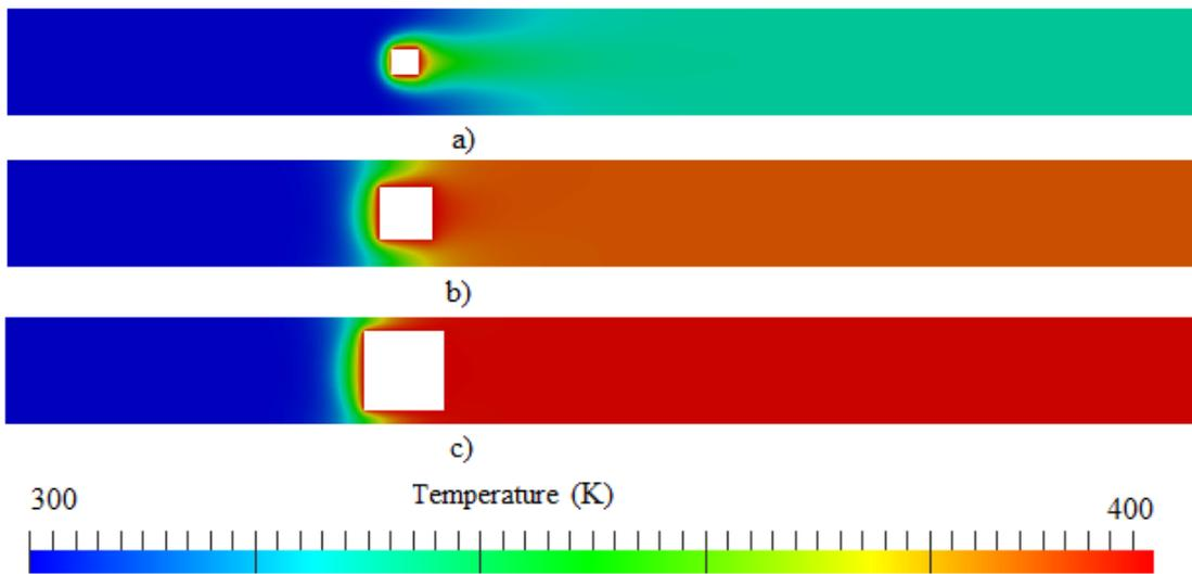
Figure 7. Temperature field for  $n = 0.4$ ,  $Pr = 10$ .
