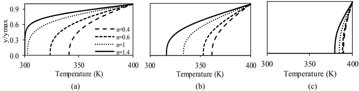
Figure 9. Temperature profile between the channel and cylinder wall,  $Pr = 10$ . (a)  $\beta = 0.25$ , (b)  $\beta = 0.5$  and (c)  $\beta = 0.75$ .
