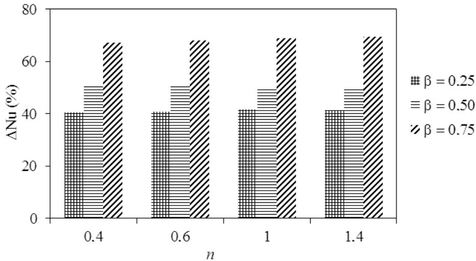
Figure 8. Variation of the Nusselt number between the numbers Prandtl 10 and 50, according to  $n$  and  $\beta$ .
