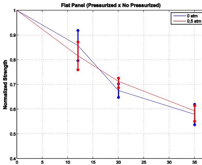
Figure 20. Flat composite laminate ( $k=0 \text{ m}^{-1}$ ) – Normalized by non impacted sample
