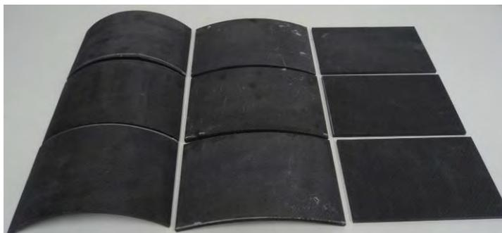
Figure 2. Manufactured samples used as reference ( $k=0.01\text{ m}^{-1}$ ,  $k=0.005\text{ m}^{-1}$ ,  $k=0\text{ m}^{-1}$ )
