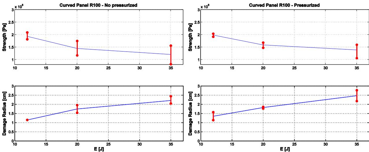
Figure 19. High curved composite laminate ( $k=0.01 \text{ m}^{-1}$ ) – Damaged radius vs Impact Energy vs Compression strength (with and without pressure)
