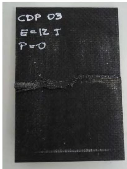
Figure 25. Flat sample after CAI ( $k=0.00 \text{ m}^{-1}$ )
