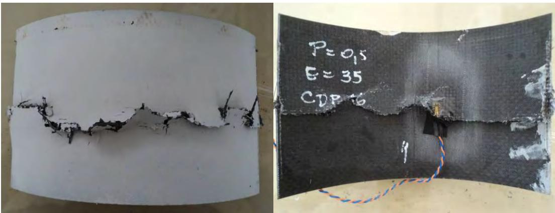
Figure 23. Curved sample after CAI ( $k=0.01\text{ m}^{-1}$ )
