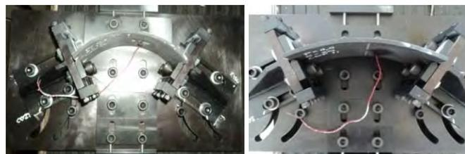
Figure 8. Different curvatures assembled on fixture ( $k=0.01\text{ m}^{-1}$ ,  $k=0.005\text{ m}^{-1}$ )
