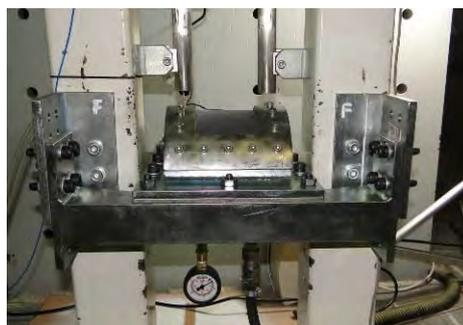
Figure 4. Impact test fixture with manometer
