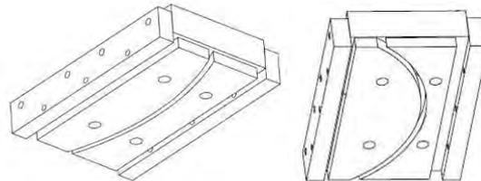
Figure 10. Upper support with different parts to hold different curvatures ( $k=0.01\ m^{-1}$ ,  $k=0.005\ m^{-1}$ )
