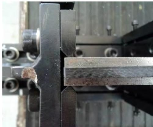
Figure 15. Boundary condition for flat samples and anti buckling system
