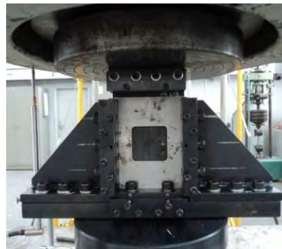
Figure 11. Fixture used to perform compression test on flat composite laminates ( $k=0\ m^{-1}$ )
