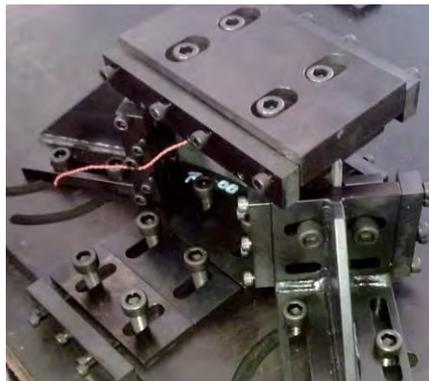
Figure 7. Fixture developed to perform compression test
