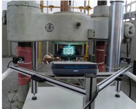
Figure 13. 3D optical system.
