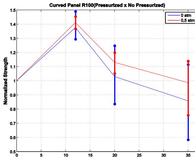
Figure 22. High curvature composite laminate ( $k=0.01 \text{ m}^{-1}$ ) – Normalized by non impacted sample
