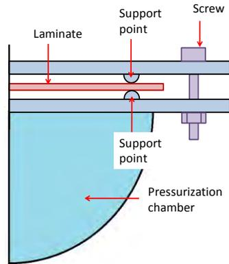
Figure 5. Pressurization system
