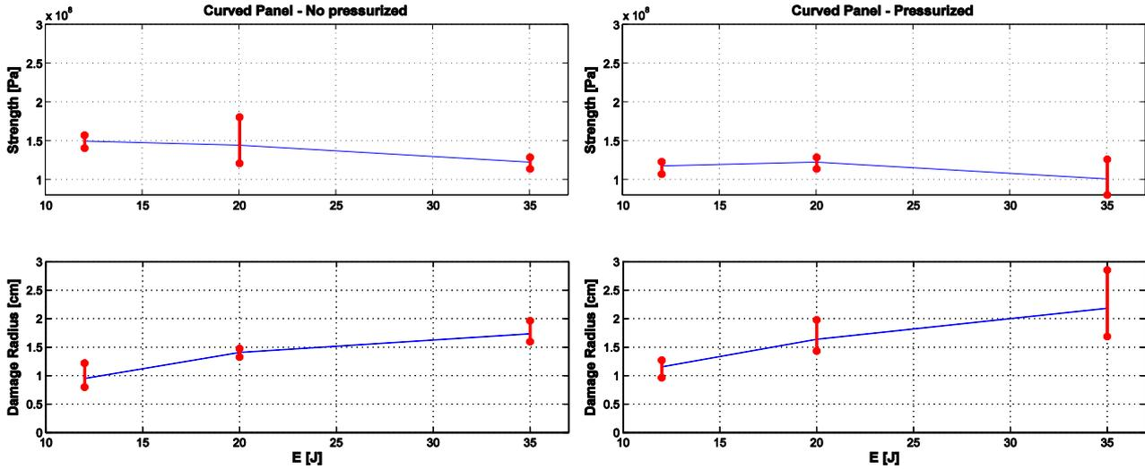
Figure 18. Medium curved composite laminate ( $k=0.005 \text{ m}^{-1}$ ) – Damaged radius vs Impact Energy vs Compression strength (with and without pressure)
