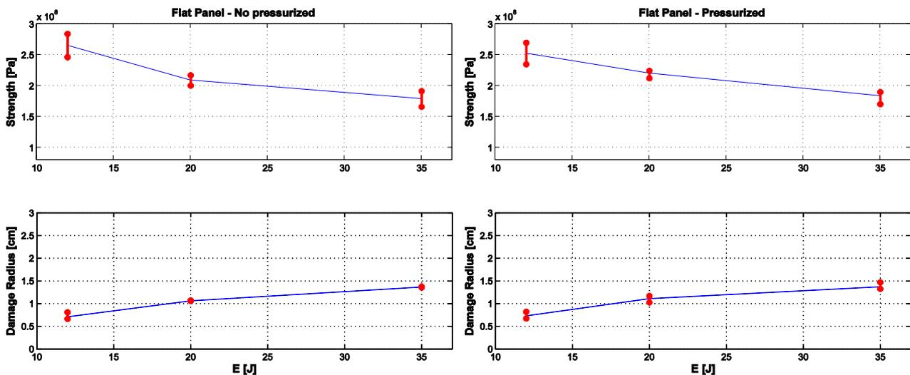
Figure 17. Flat composite laminate ( $k=0\text{ m}^{-1}$ ) – Damaged radius vs Impact Energy vs Compression strength (with and without pressure)
