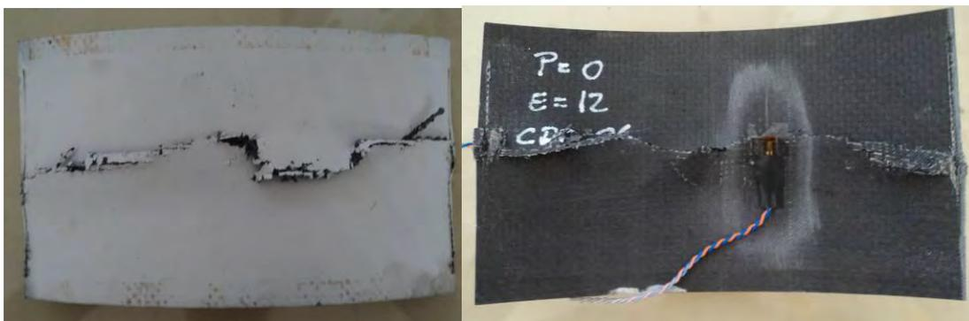
Figure 24. Curved sample after CAI ( $k=0.005\text{ m}^{-1}$ )
