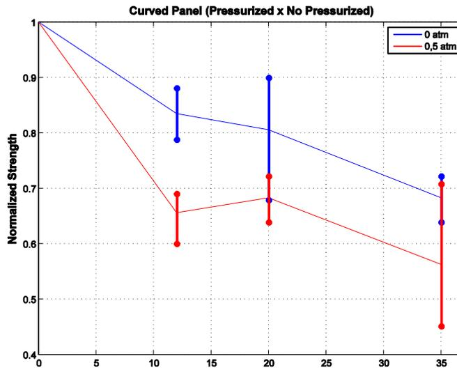
Figure 21. Medium curvature composite laminate ( $k=0.005 \text{ m}^{-1}$ ) – Normalized by non impacted sample
