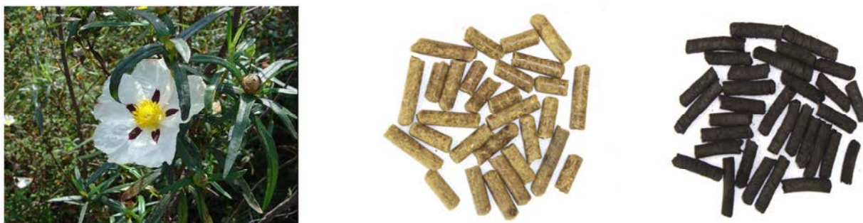
Figure 1 – Cistus shrub (left); Cistus pellets, before and after carbonization (center and right).
