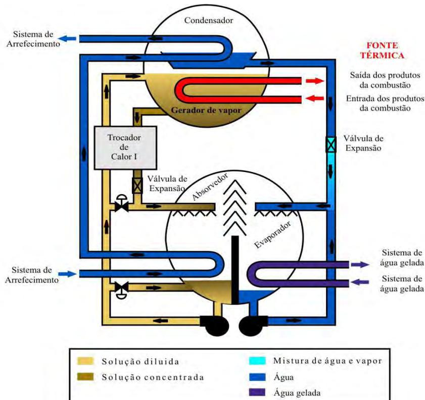
Figure 2. Diagram of absorption cooling system of simple effect with pair water - lithium bromide.
