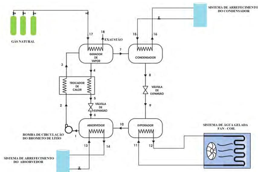
Figure 3. Schematic of the absorption cooling system of simple effect created in IES - UFPB with their own points of entry and exit.
