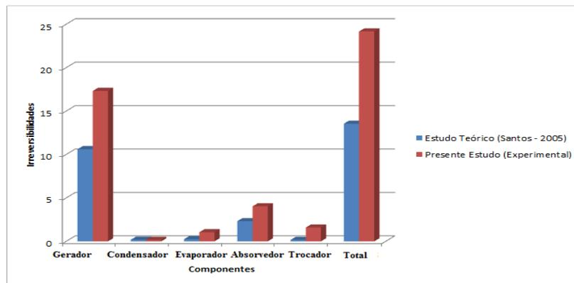
Figure 11. Comparison of the irreversibility of each component in addition to the full.
