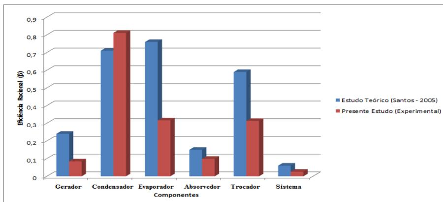
Figure 10. Rational comparison of the efficiency of each component.
