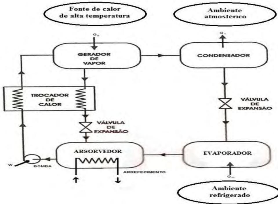
Figure 1. Simplified schematic of absorption cooling system of simple effect.
