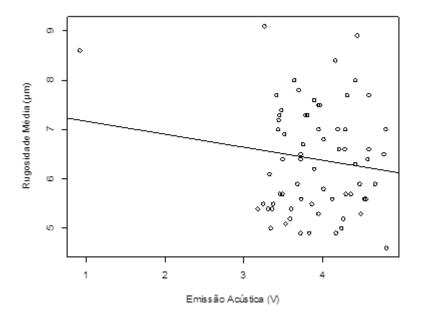
Figure 5 - Graph of linear regression for the average roughness (Ra) as a function of acoustic emission in the sanding of *Corymbia citriodora*.
