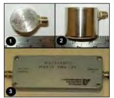
Figure 3 - Module Acoustic emission (1) sensor (2) and amplifier (3).
