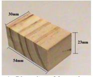
Figure 1 - Dimensions of the specimens.
