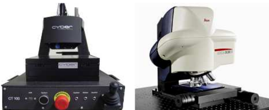
Figure 5 - Chromatic aberration confocal microscope (left); Conventional confocal microscope (right)
