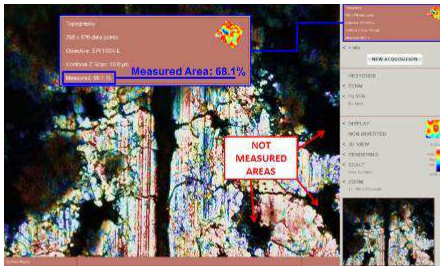
Figure 6 - Image quality verification with measured area criterion
