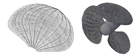
Figure 12.(a) Details of the blade designed. (b) Propeller 3 blade designed in 3D.
