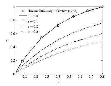
Figure 5. Efficiency location relative to the advance coefficient location.
