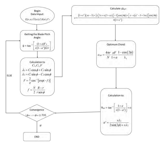
Figure 3. Routine to obtain Chord and Twist Angle, without considering cavitation effect.
