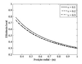
Figure 11.Local propeller efficiency as a function of radial position for each blade element.
