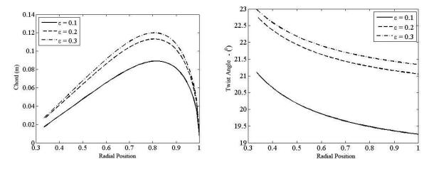
Figure 9. (a) Distribution of chord and (b) distribution of the blade twist angle on propeller.
