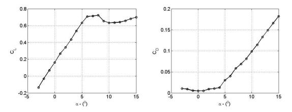
Figure 7. (a) Lift coefficient and (b) drag coefficient as a function of angle of attack for the hydrodynamic profile NACA 66206 (Abbot *et al*, 1959)- Reynolds 5x10<sup>5</sup>.
