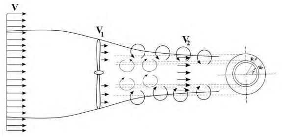
Figure 1. Illustration of the stream around propeller.
