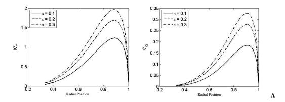
Figure 10. (a) Local thrust coefficient  $(k_0^*)$  and (b) Local torque coefficient  $(k_T^*)$  as a function of radial position.
