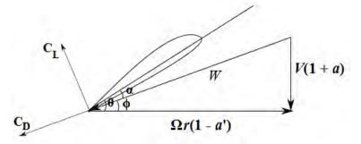
Figure 2.Forces and velocities acting on a section of the blade.
