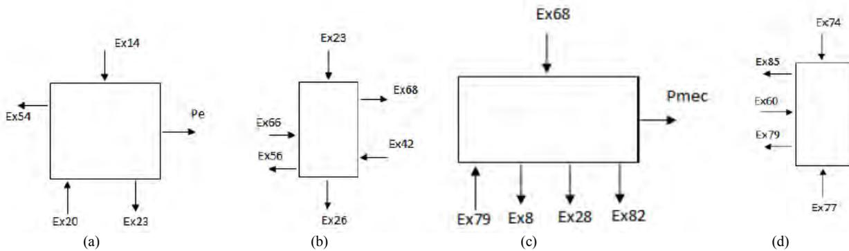
Figure 7 – Black-box for (a) gas turbine, (b) heat recovery steam generator, (c) steam turbine and (d) biomass boiler
