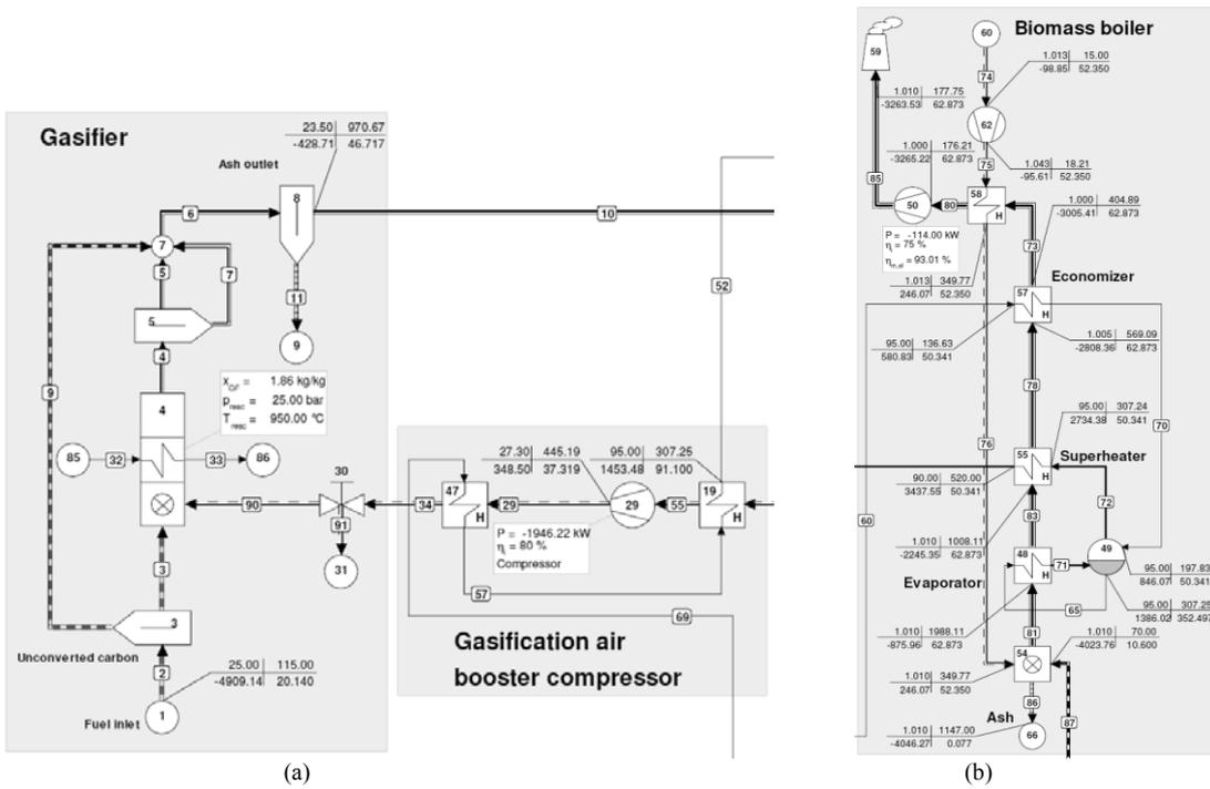
Figure 4: (a) Gasifier and gasification air booster compressor; (b) Biomass boiler
