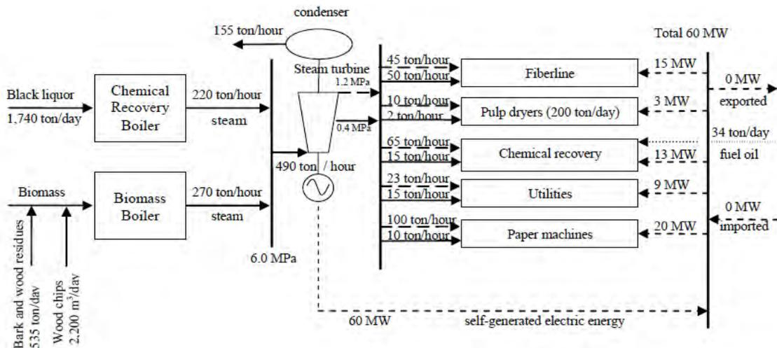
Figure 2 - Integrated pulp and paper mill with extraction/condensing cogeneration scheme (adapted from Moraes, 2011)
