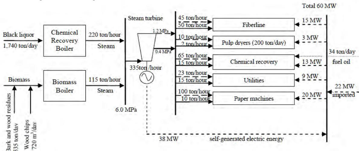
Figure 1 - Integrated pulp and paper mill with backpressure/extraction cogeneration scheme (adapted from Moraes, 2011)
