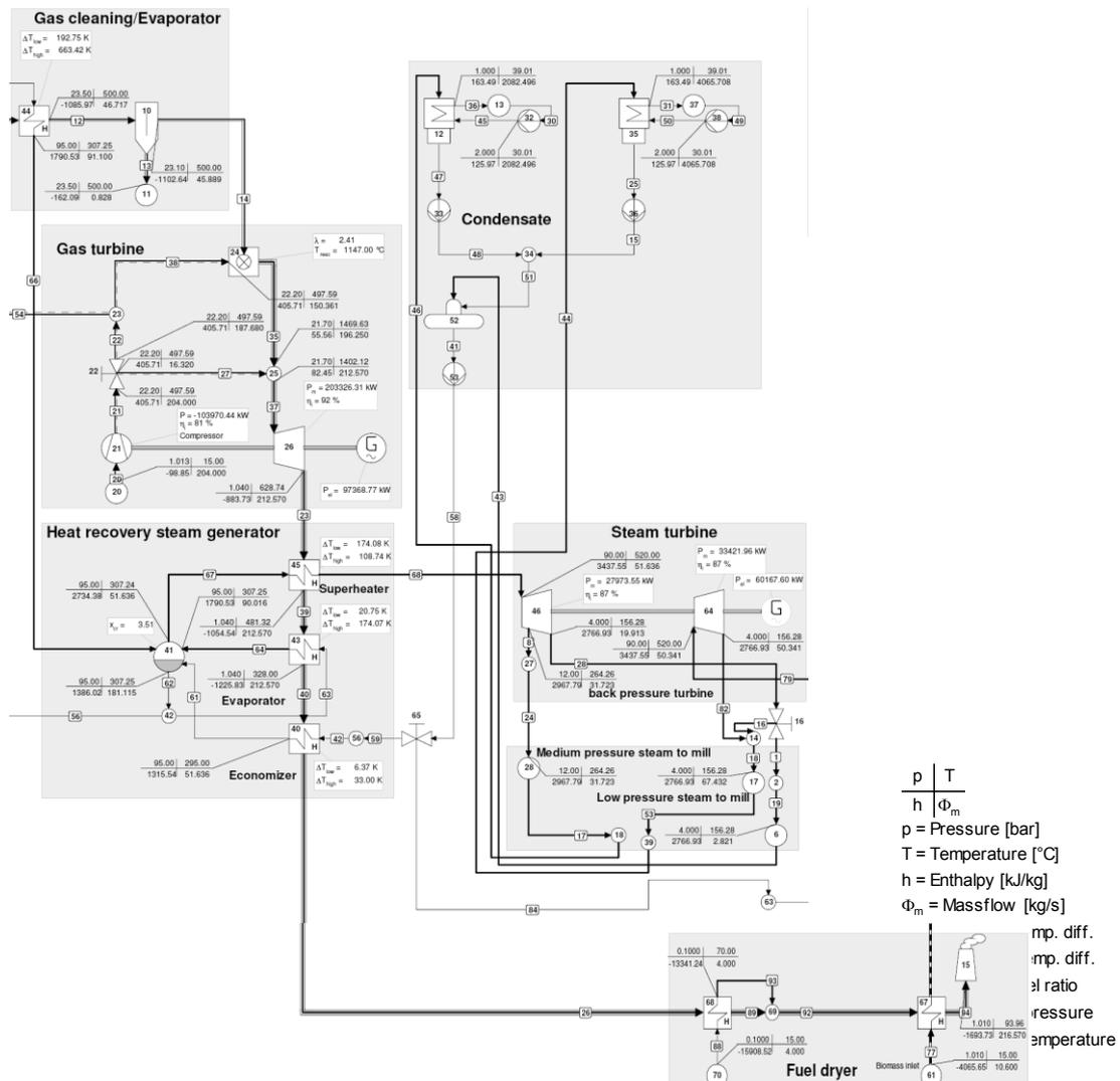
Figure 5: Gas turbine, HRSG and steam turbine.
