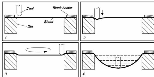
Figure 03. Single point incremental forming scheme (Kim, 2000, cited in Pohlak, 2007)
