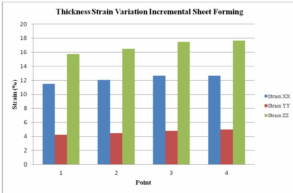
Figure 13: Strain variation along thickness in Incremental Stamping
