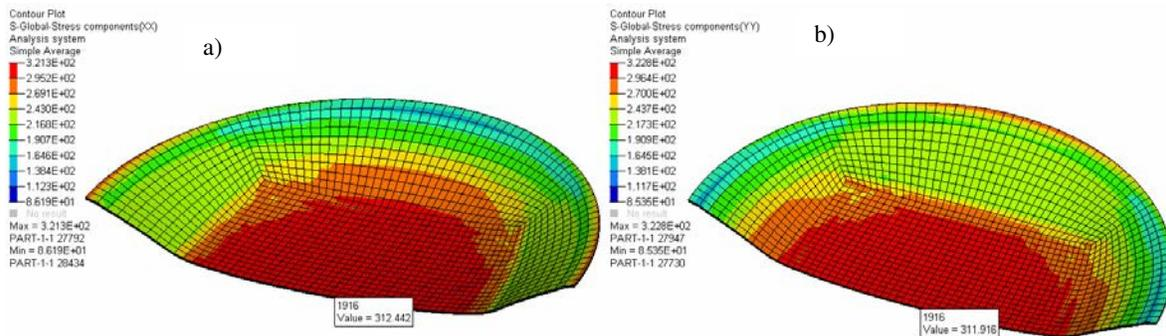
Figure 08: Conventional Stamping a)  $\sigma_{xx} = 312.442$  MPa, b)  $\sigma_{yy} = 311.916$  MPa
