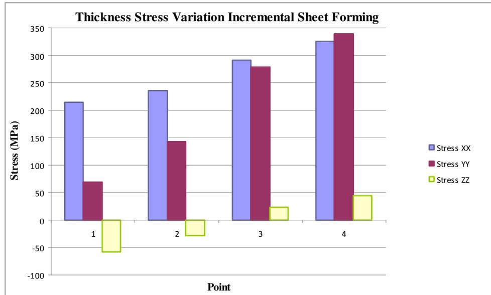
Figure 11: Stress variation along thickness in Incremental Stamping
