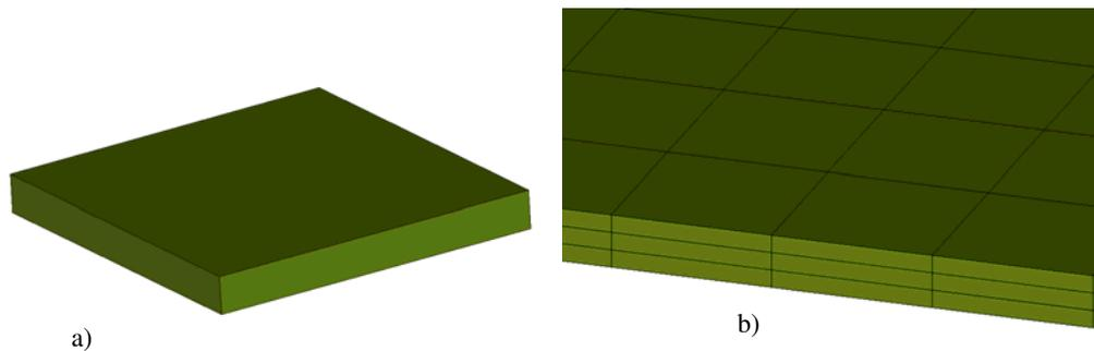
Figure 05: FEM Model a) 8 nodes elements, b) Elements configuration along the thickness
