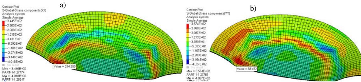
Figure 09: Incremental Stamping a)  $\sigma_{xx} = 214.255$  MPa, b)  $\sigma_{yy} = 68.452$  MPa
