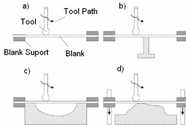
Figure 02. Kinds of Incremental Stamping a) Single point incremental forming; b) double point incremental forming; c) with negative die; d) with positive die (Castelan, 2007)
