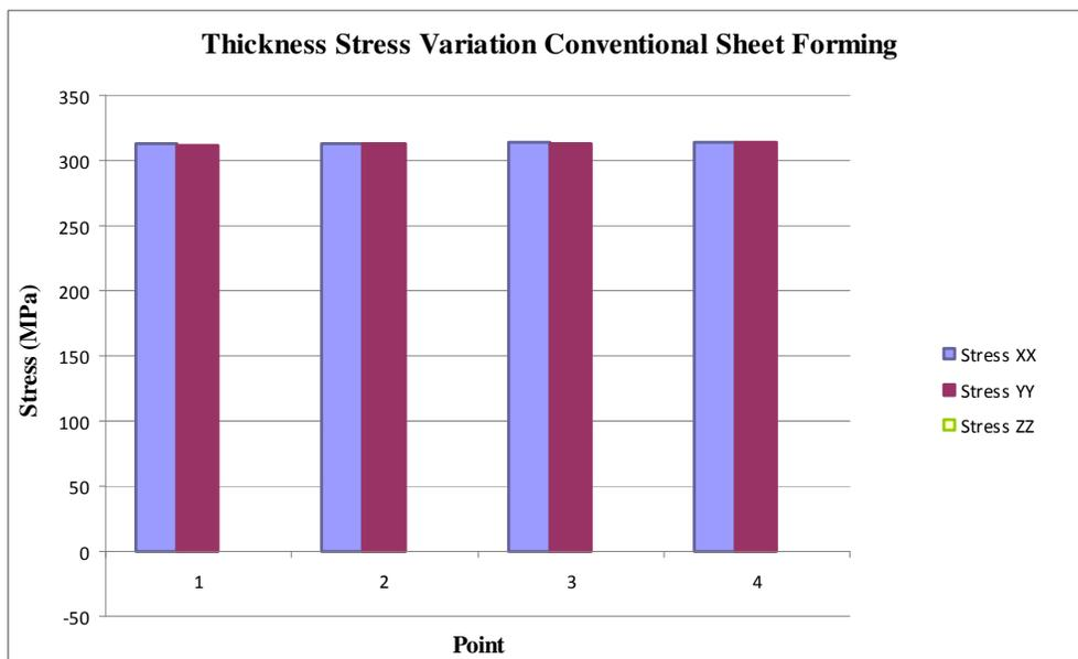
Figure 12: Stress variation along thickness in Conventional Stamping
