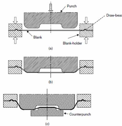
Figure 01: Conventional Stamping a) blank and tools position b) punch acting on the blank, c) contact between blank and die (Marciniak *et al*, 2002)
