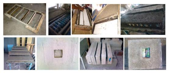
Figure. 2. Manufacturing steps of blocks with three fillings used.
