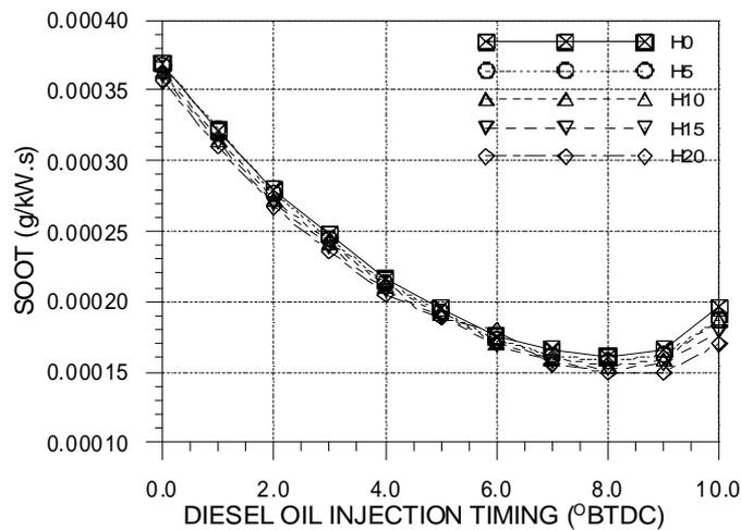
Figure 4. Soot emissions with advancing injection timing and different amounts of hydrogen
