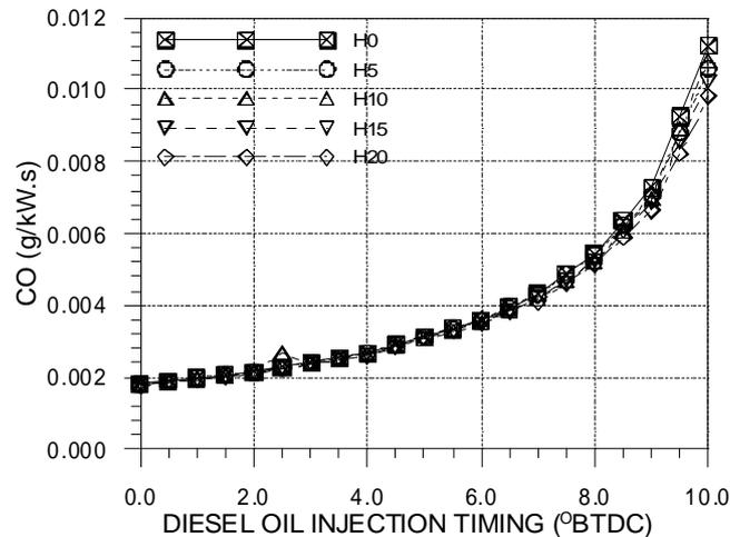
Figure 3. CO emissions with advancing injection timing and different amounts of hydrogen
