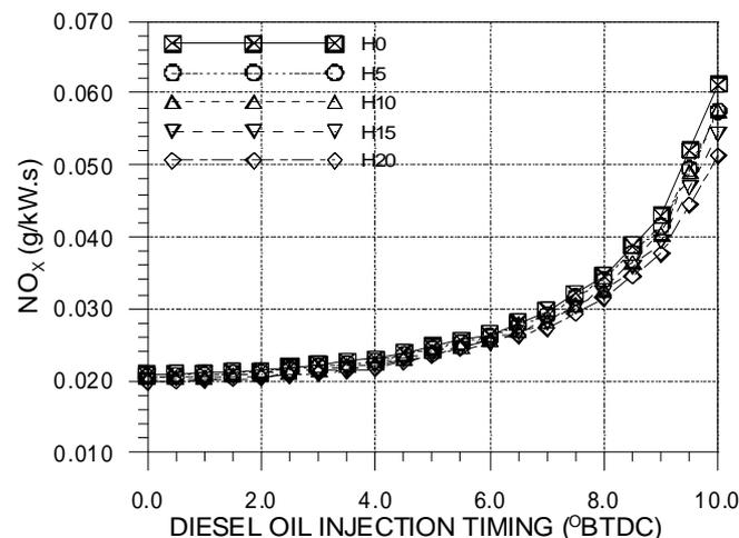
Figure 2.  $\text{NO}_x$  emissions with variation of injection timing and hydrogen amount
