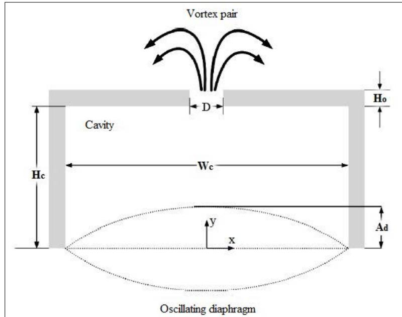
Figure 1. Schematic of a piezoelectrically driven synthetic jet cavity geometry and its dimensions.
