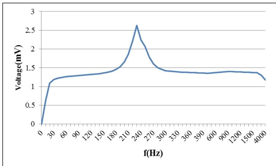
Figure 5. Natural diaphragm frequency measurements.
