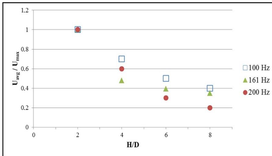
Figure 7. Normalized average speed ( $U_{avg}/U_{max}$ ) at distances  $H/D=0$  to 8 with a 20 x 5 mm rectangular orifice (Configuration 1) for three frequencies.
