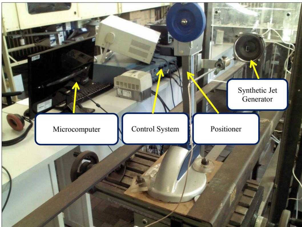
Figure 3. Equipments used for calibration and testing of the synthetic jet generator.
