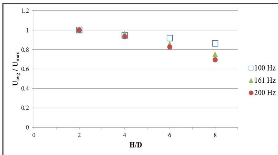
Figure 8. Normalized average speed ( $U_{avg}/U_{max}$ ) at distances  $H/D=0$  to 8 with a 10 x 2.5 mm rectangular orifice (Configuration 2) for three frequencies.
