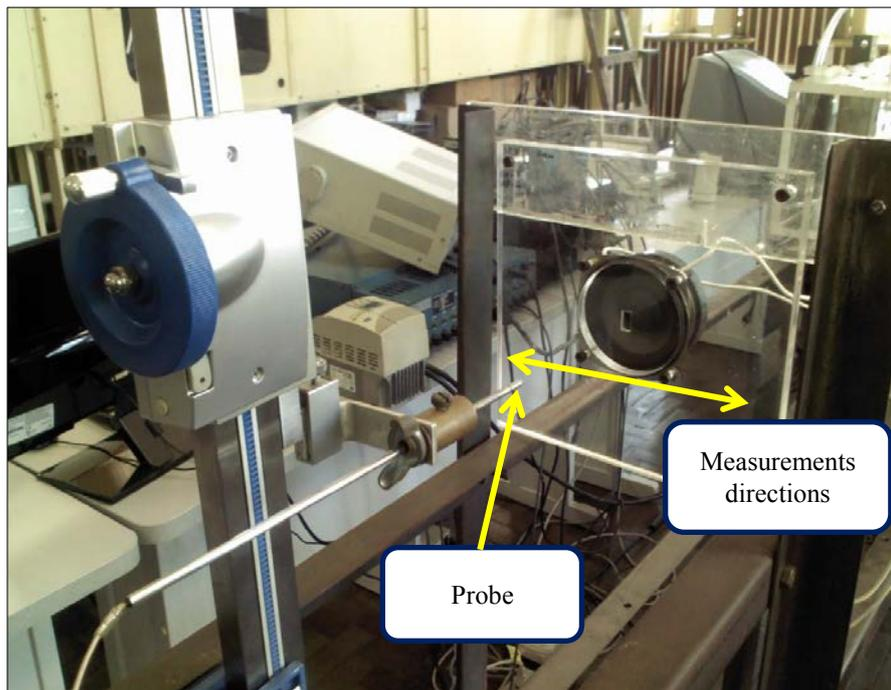
Figure 11. Test section with hot-wire anemometer for mapping the jet width.
