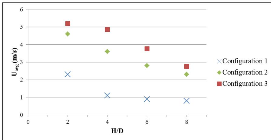
Figure 10. Average speed at distances  $H/D=0$  to 8, for all three configurations with the optimal frequency of 161 Hz.
