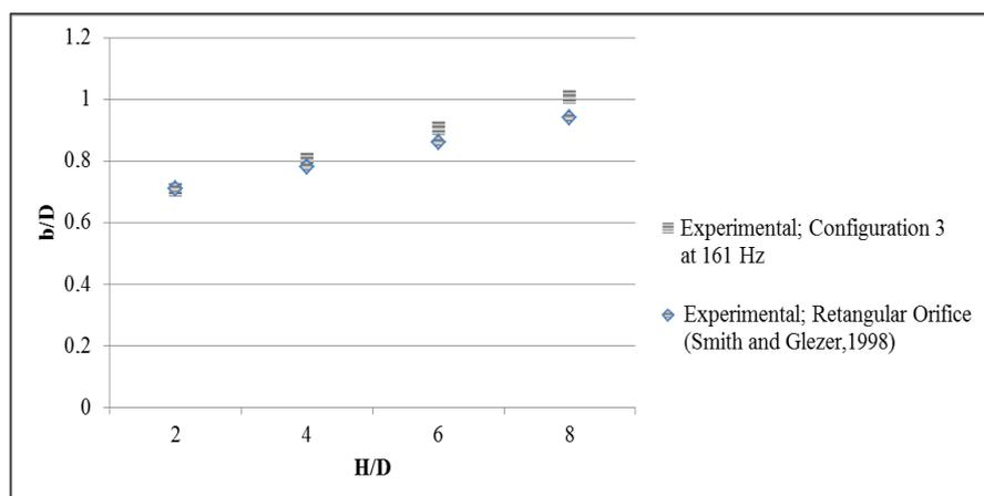
Figure 12. Average width of the jet ( $b/D$ ) vs. axial distance ( $H/D$ ) for rectangular orifice with dimensions of 12 x 6 mm (Configuration 3) at optimal frequency compared to the study of Smith and Glezer (1998).
