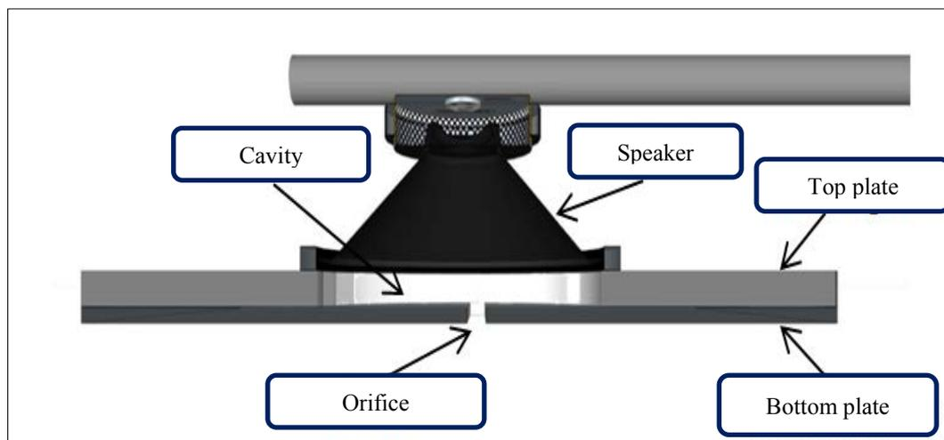
Figure 2. Schematic of the synthetic jet generator manufactured for this study.
