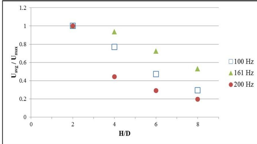
Figure 9. Normalized average speed ( $U_{avg}/U_{max}$ ) at distances  $H/D=0$  to 8 with a 12 x 6 mm rectangular orifice (Configuration 3) for three frequencies.
