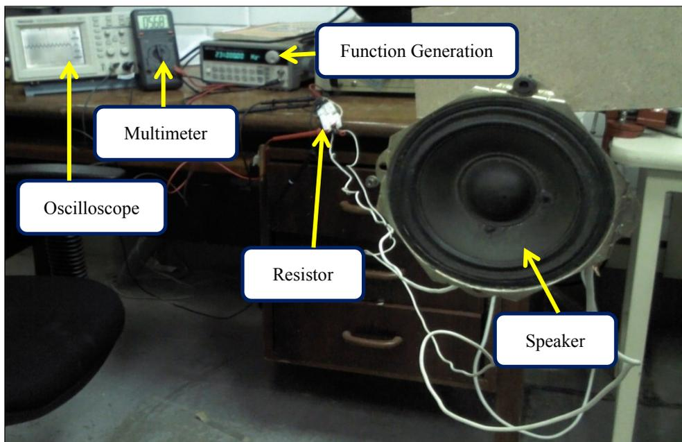
Figure 4. Speaker mounting for measuring the resonance frequency outdoors.
