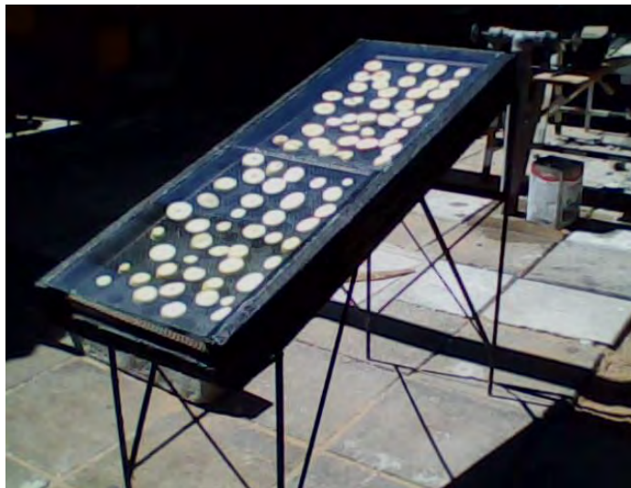
Figure 3. Already built equipment drying apples and pears
