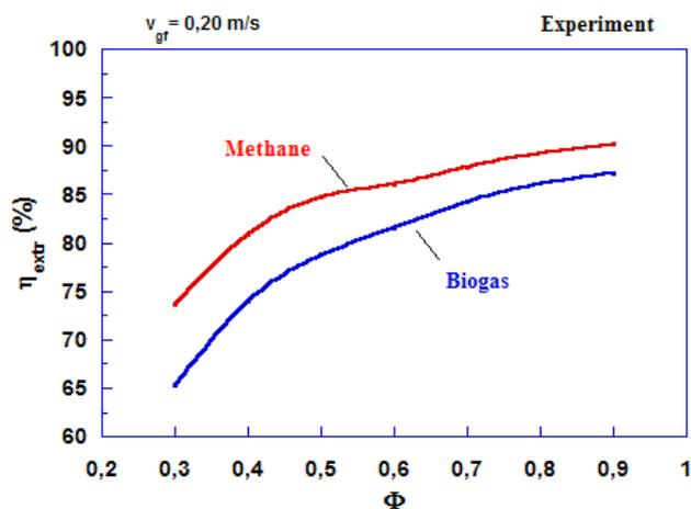
Figure 6 – Energy extraction efficiency for both the study fuels: methane & biogas ( $v_{gr} = 0,2$  m/s)
