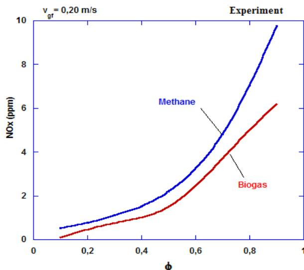
Figure 7 – NO<sub>x</sub> emission profiles for both the study fuels: methane and biogas ( $v_{gr} = 0,2$  m/s)
