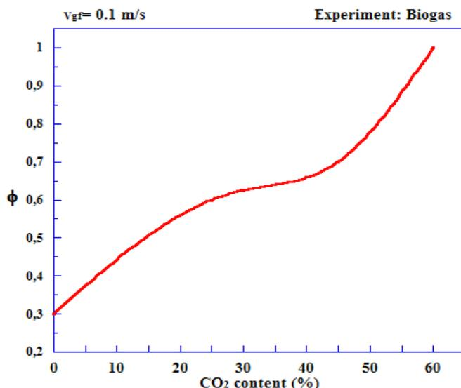
Figure 9 - Flammability limit for unidirectional flow porous burner as a function of  $\text{CO}_2$  content ( $v_{gf} = 0.1$  m/s)
