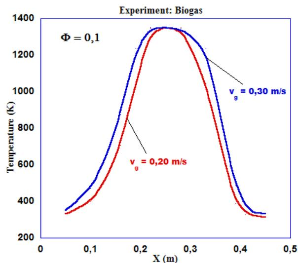
Figure 2 – Temperature distribution profile, varying  $v_{gf}$  with constant equivalence ratio ( $\Phi = 0.10$ .)
