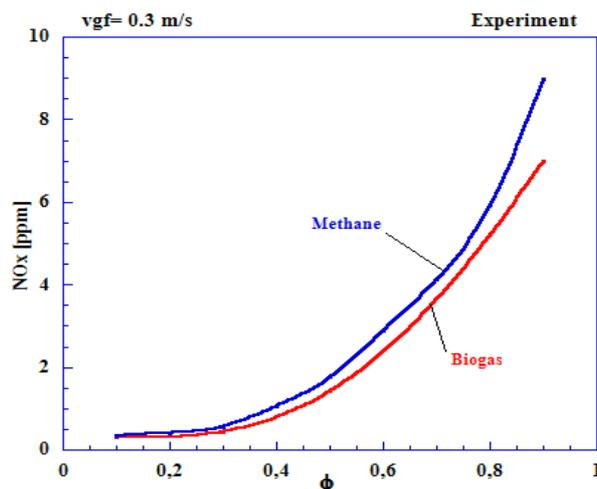
Figure 8 -  $\text{NO}_x$  emission profiles for both the study fuels: methane and biogas ( $v_{gf} = 0.3$  m/s)
