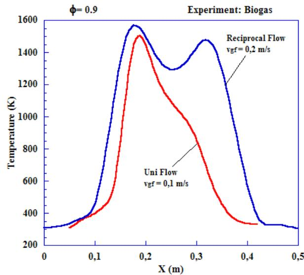
Figure 4 – Temperature distribution profile of biogas: reciprocal & unidirectional flows
