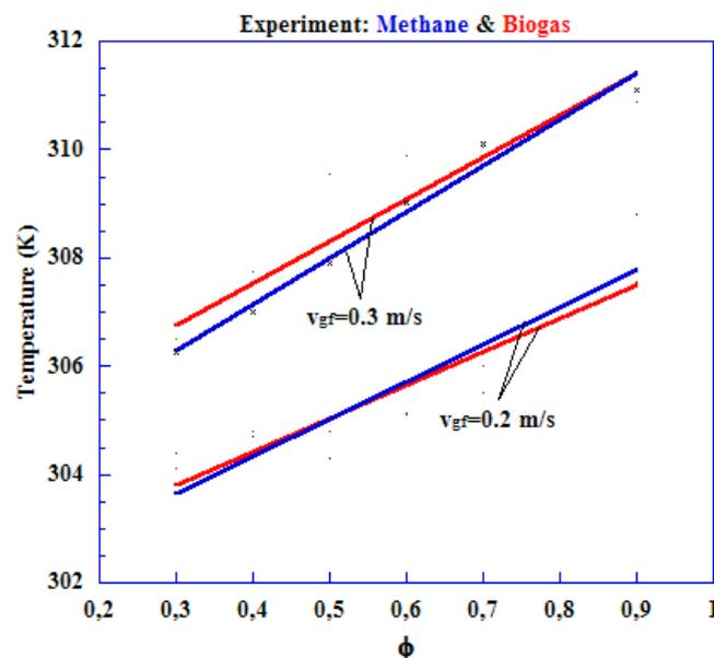
Figure 5 – Exhaust temperature on reciprocal flow for both the reference gases: methane & biogas
