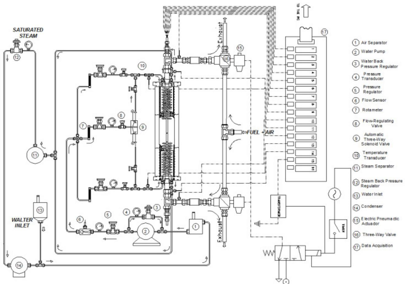
Fig. 1 – Reciprocating flow porous burner with its supply and control systems
