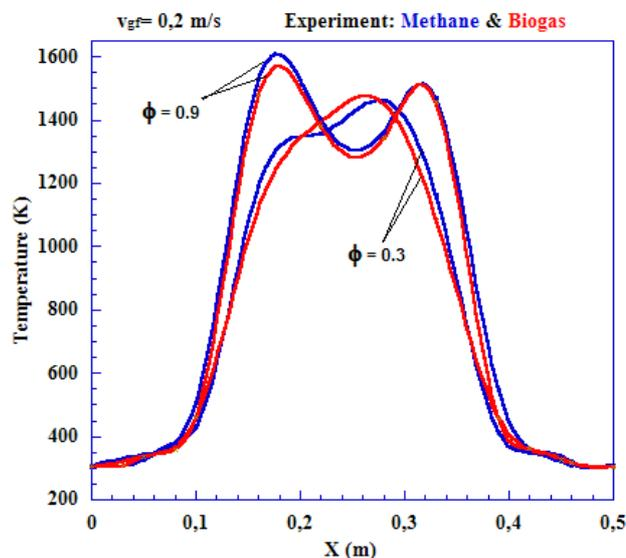
Figure 3 – Temperature distribution profiles: methane & biogas, varying “ $\Phi$ ” from 0.30 to 0.9 with  $v_{gf}=0.20$  m/s
