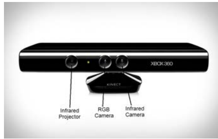
Figure 2. Kinect camera. Depth resolution: 640 \times 480 px, RGB resolution: 1600 \times 1200 px.
