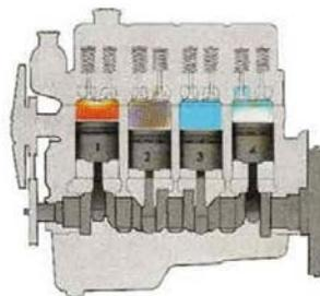
Figure 3. Operating cycles of combustion engine four-stroke and four-cylinder
