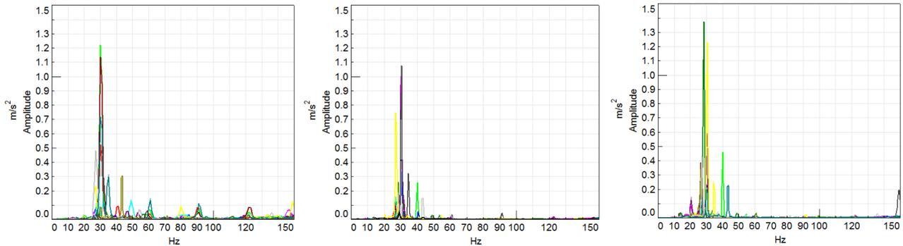
Figure 17. X, Y and Z direction vibration spectral analysis
