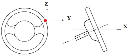
Figure 15. Direction of vibration during the study
