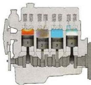
Figure 3. Operating cycles of combustion engine four-stroke and four-cylinder
