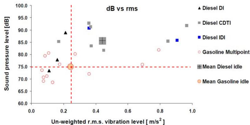
Figure 8. Analysis of sound pressure as a function of steering wheel vibration measured on 24 cars in idle condition (source:(Ajovalasit & Giacomini, 2008))
