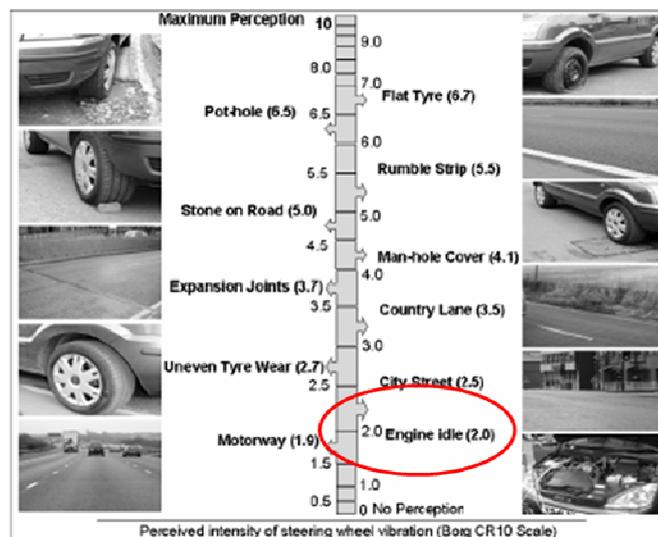
Figure 6. Proposal of subjective assessment scale to quantify the perceived vibration intensity at the steering wheel in various conditions of use of vehicle (source: (Giacomin & Gananasekaran, 2005)).
