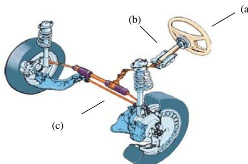
Figure 2. Vehicular steering system (a) wheel, (b) the steering column and (c) steering box
