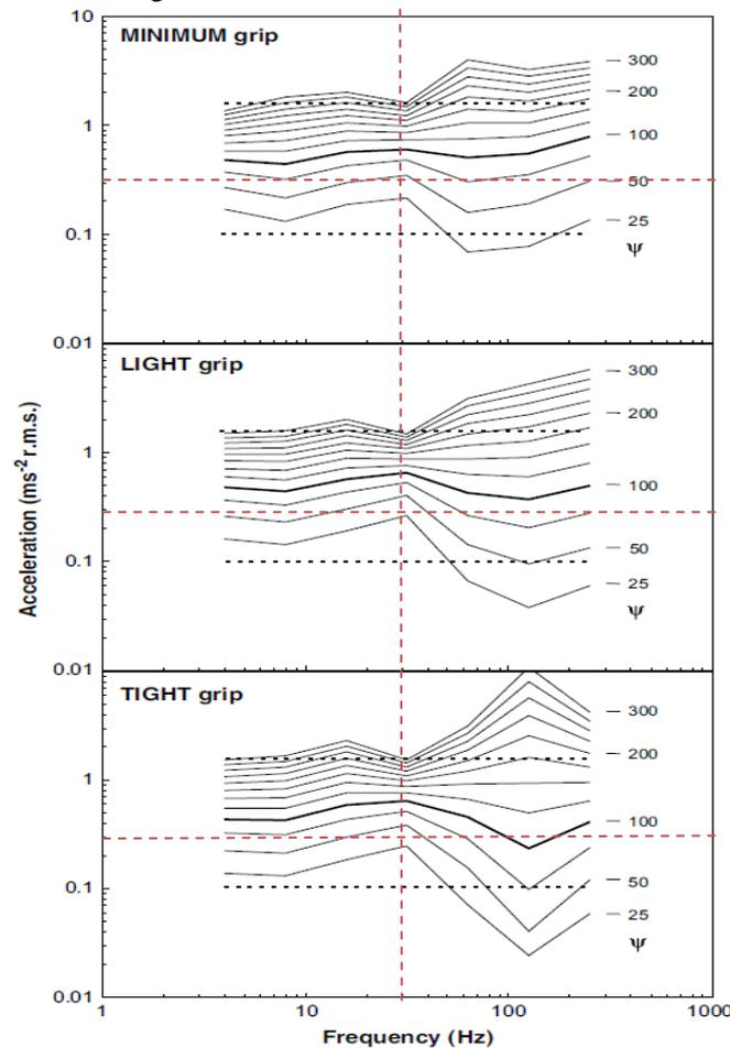
Figure 13. Equivalent comfort contours amplitudes for each of the three hands' grip force (source: (Morioka & Griffin, 2009))
