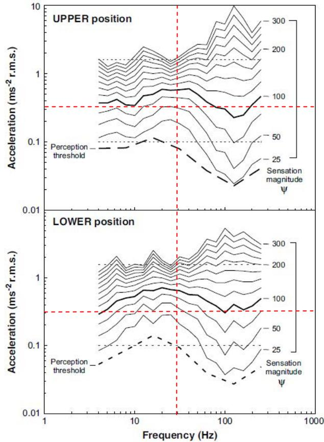
Figure 10. Equivalent comfort contours for each of the two hand positions (source: (Morioka & Griffin, 2009))
