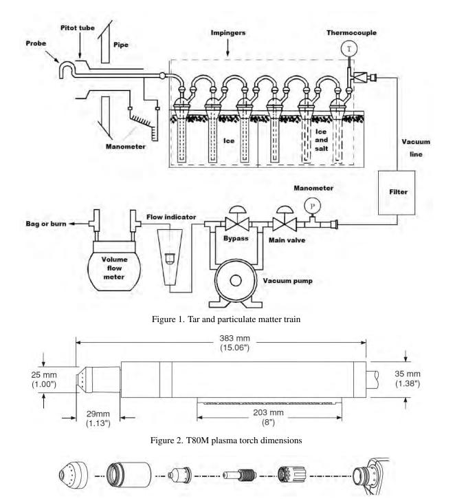
Figure 3. Scheme of installation of consumables for gouging. From left to right: nozzle protection, retention nozzle, nozzle, electrode, gas distributor and nozzle coupling torch
