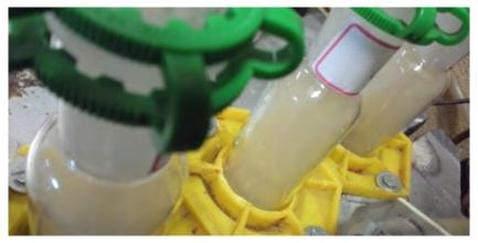
Figure 7. Pyrolysis gas inside the impingers
