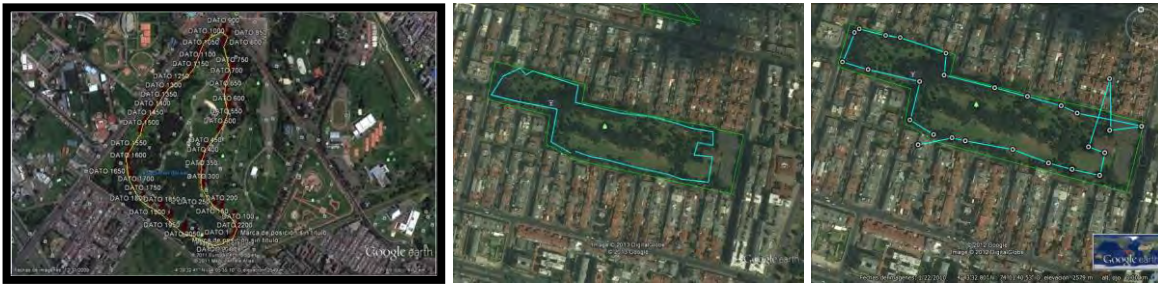
Figure 2. – Representation in Google Earth GIS data taken at Simon Bolivar Park in Bogota, Colombia (left side) with GPS Geo Explorer 3 and Cedro Salazar Park with Geo Explorer 3 in average precision (center) and Dexter dGPS (right side). (Google Earth Version 6.0.1.2032 - beta).
