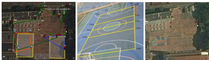
Figure 1 – Images measurement data of La Salle University in Bogota, with GPS MAP 60CSx (left), sports field points measured with Geo Explorer 3 (center) and the same points represented in the GIS Google Earth (right). (Google Earth Version 6.0.1.2032-beta).
