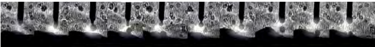
Figure 8. Spray transfer mode.
