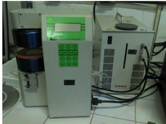
Figure 12. LaserComp Fox-50 and the heat exchanger
