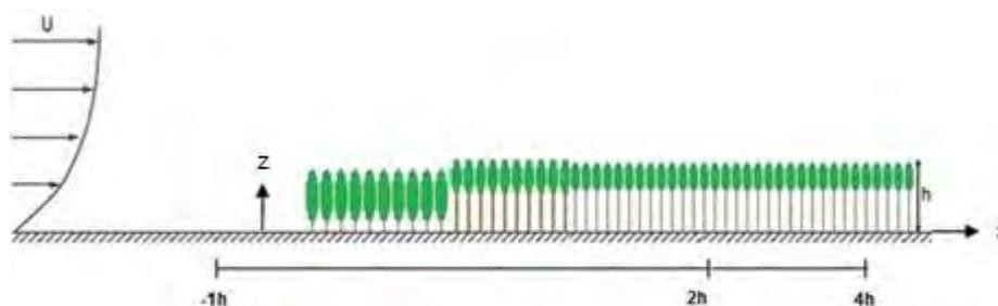
Figure 11. Side view: Schematic representation of WTF5: windward structure formed with trees types T2 and T4.
