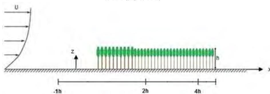
Figure 5. Side view: Schematic representation of WTF2: windward structure formed with trees type T2.
