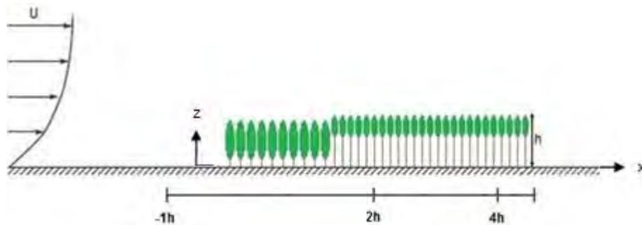
Figure 9. Side view: Schematic representation of the WTF4: windward structure formed with trees types T4.
