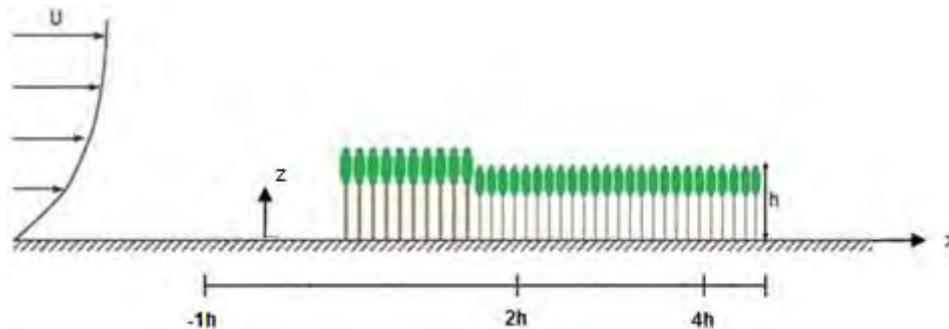
Figure 7. Side view: Schematic representation of WTF3: windward structure formed with trees type T3.
