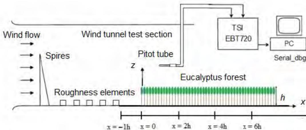
Figure 1. Sketch of the wind tunnel test section, measurement system and homogeneous forest localization.
