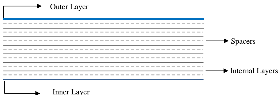
Figure 1 - Schematic representation of a MLI blanket
