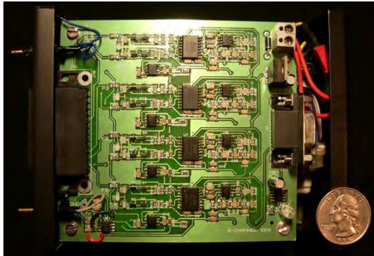
Figure 2. Miniaturized embedded version of the developed 8-channel electroencephalograph, used in the experiments.
