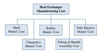
Figure 1. Scheme of heat exchanger manufacturing cost decomposition.
