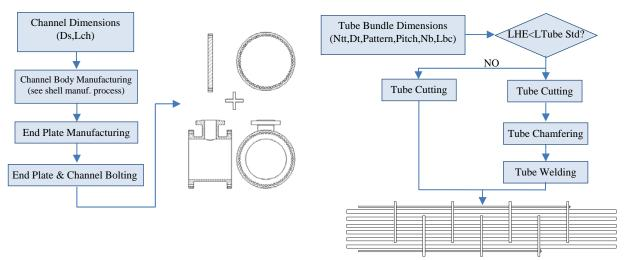
Figure 4. Scheme of tube sheet manufacturing process.
