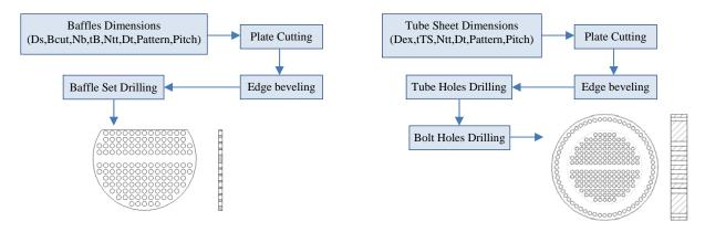
Figure 2. Scheme of baffle manufacturing process.
