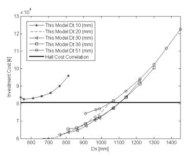
Figure 6. Sensitivity of exchanger cost to changes of geometrical architecture.
