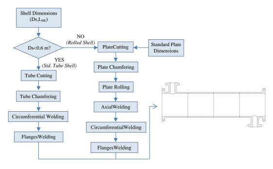
Figure 1. Scheme of shell manufacturing process.
