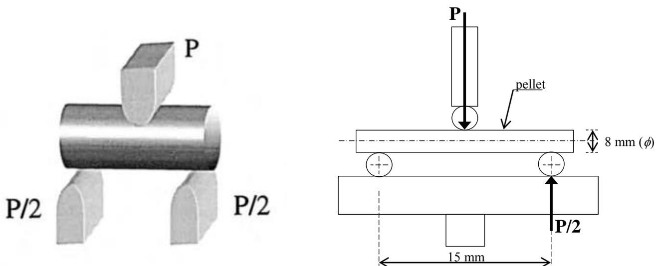
Figure 4. Experimental set-up scheme, pellets testing machine.
