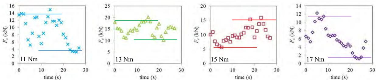
Figure 13. Range of maximum and minimum compression forces during *Salix* pellets manufacturing.
