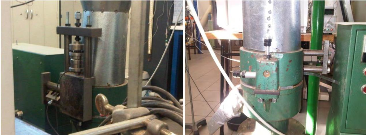
Figure 2. Experimental set-up, pelletizer machine: load cells and axis adjustments.
