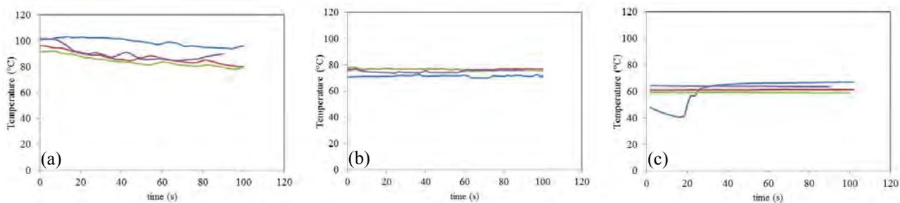
Figure 6. *Acacia* temperature versus time for different initial tightening torques: (a) axis, (b) upper cover, (c) lower tub. (violet, 11; green, 13; red, 15; blue 17 Nm).
