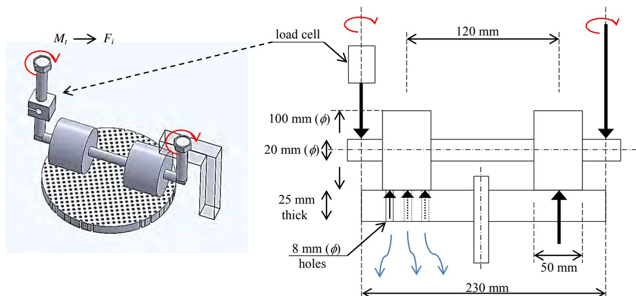
Figure 1. Experimental set-up schemes, pelletizer machine.
