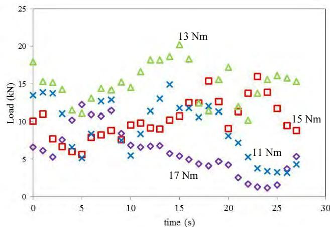
Figure 12. Compression forces ( $F_c$ ) obtained during manufacturing of *Salix atrocinerea* pellets at constant temperature.
