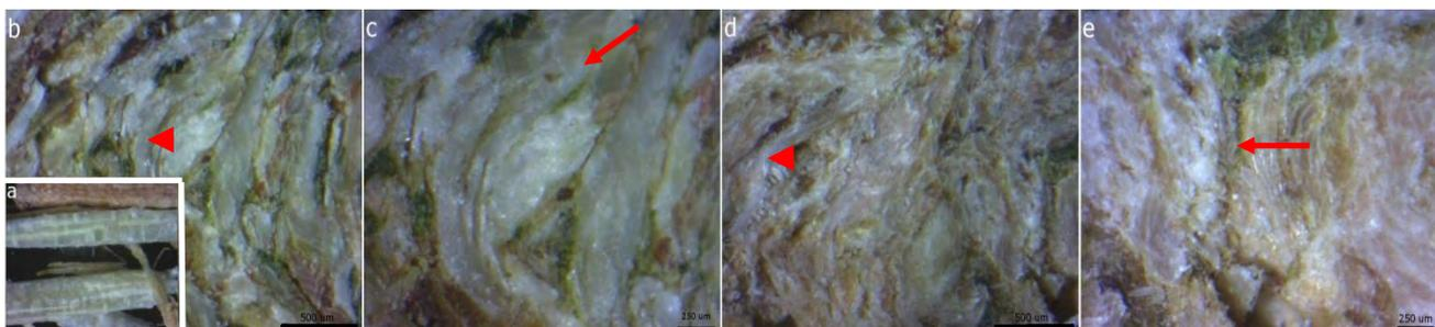
Figure 11. Wood particles and longitudinal cross sections of pellets. Image (a) presents wood particles before pelletization. Images (b) and (c) show longitudinal cross sections of *Acacia* while images (d) and (e), corresponding to the longitudinal cross section of *Salix* pellets, show bended and oriented particles.
