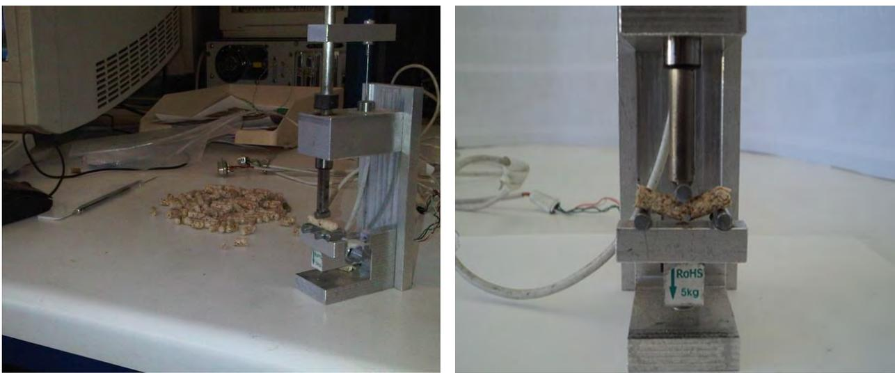
Figure 5. Experimental set-up and photograph of fracture pieces.
