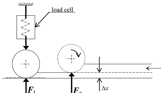
Figure 3. Initial (static) and final deformation of the plate/load cell set.
