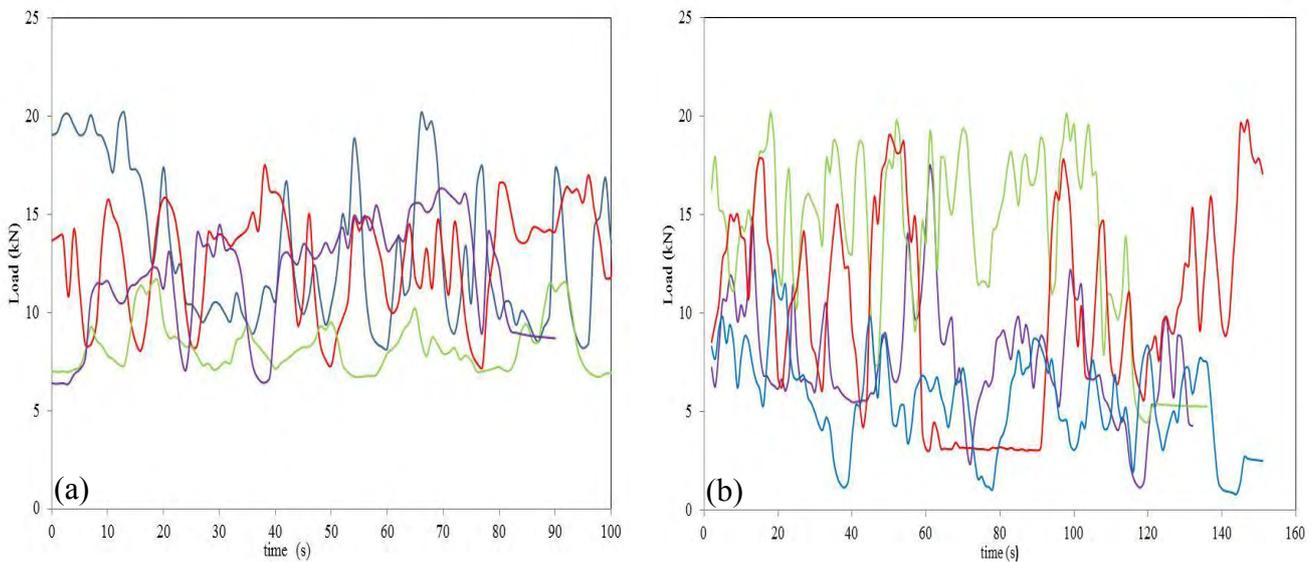
Figure 8. Vertical force values *versus* time for different initial tightening torques: (a) *Acacia*, (b) *Salix*. (violet, 11; green, 13; red, 15; blue 17 Nm).
