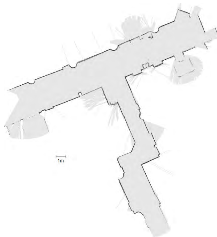
Figure 9. Resulting map after the application of DP-SLAM on the data from Figure 7.
