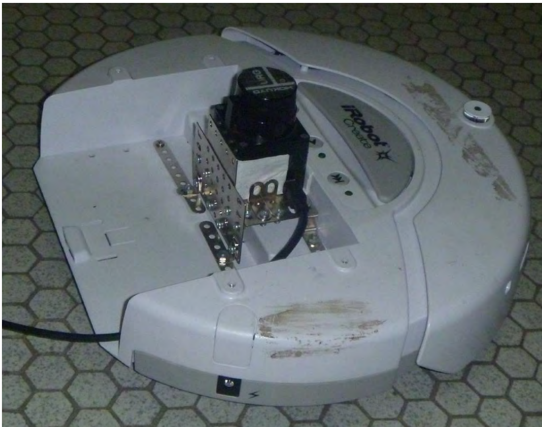
Figure 3. Mobile robot iRobot Create coupled with the Laser Range Finder.
