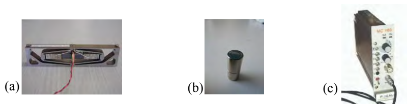
Figure 2. (a) Amplified Piezoelectric Actuator – APA. (b) Capacitive sensor. (c) Converter module.
