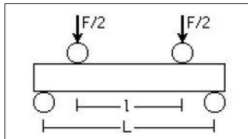
Figure 2. Schematic test at four points
