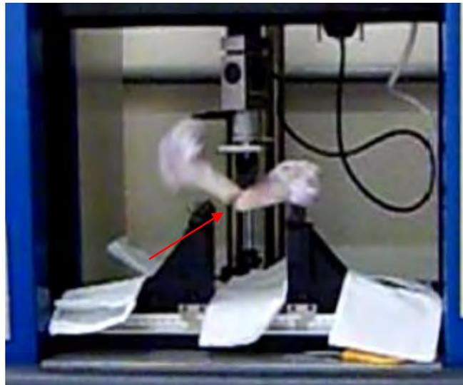
Figure 7. Photographic image of the bone being fractured. Note the arrow to the failure occurring by traction
