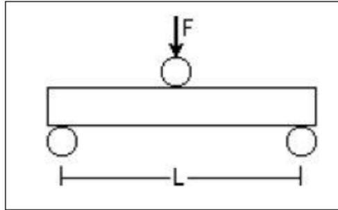
Figure 1. Schematic test at three points.
