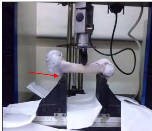
Figure 3. Photographic image of the bending test. Note the arrow to the bone (femur pig) supported with span of 100 mm
