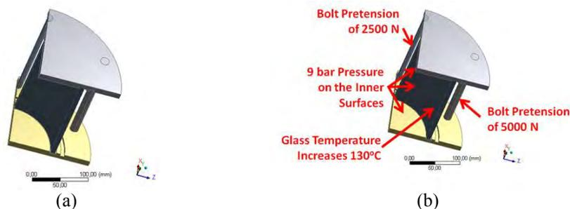
Figure 3. Static structural simulation (a) the test rig model, (b) the boundary conditions.
