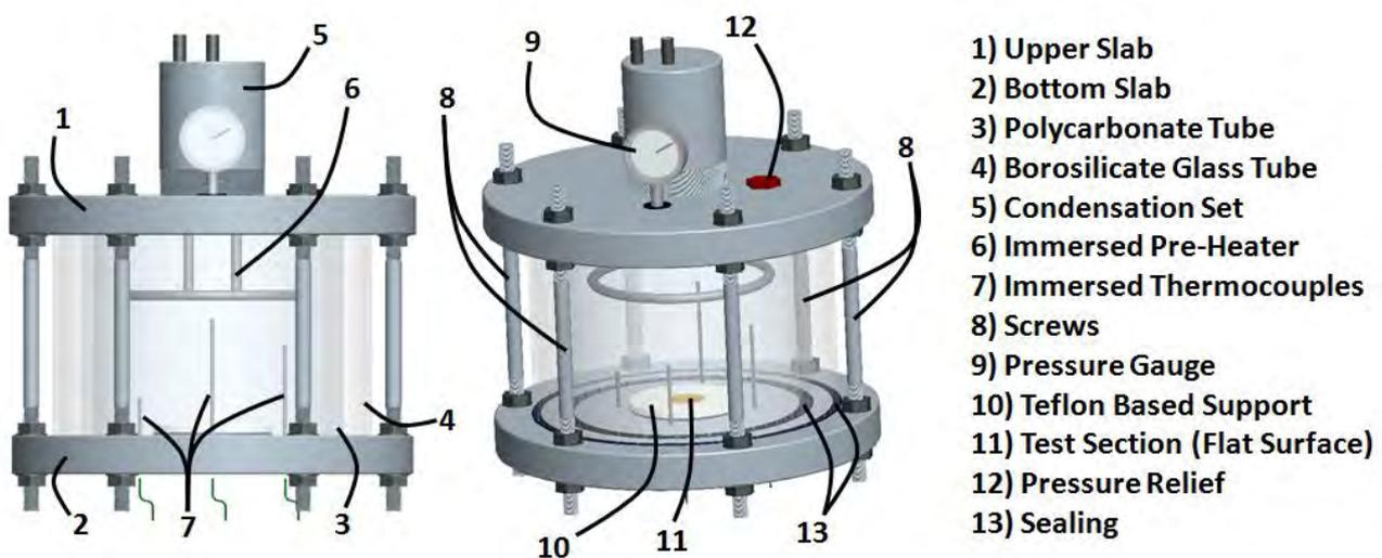
Figure 2. Nucleate pool boiling test rig developed for high pressures and high temperatures
