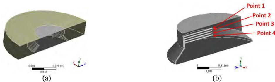
Figure 4. Test section thermal simulation (a) the test section set, (b) the test section model.
