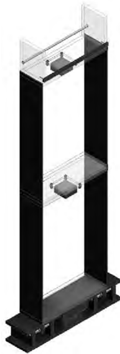
Figure 3. Reduce Scale Model of Two-floor building.
