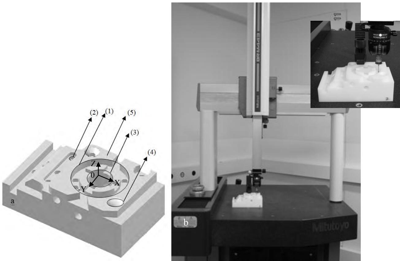
Figure 1 - Measured part (a) and Coordinate Measurement Machine used in the experiments (b)
