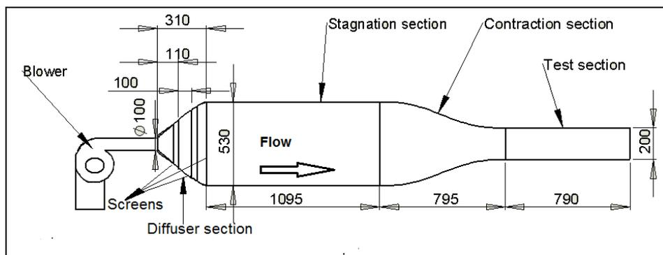
Figure 1. Schematics of the low-speed wind tunnel
