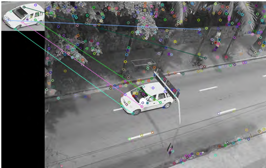
Figure 7: Tracking the vehicle with SIFT algorithm only
