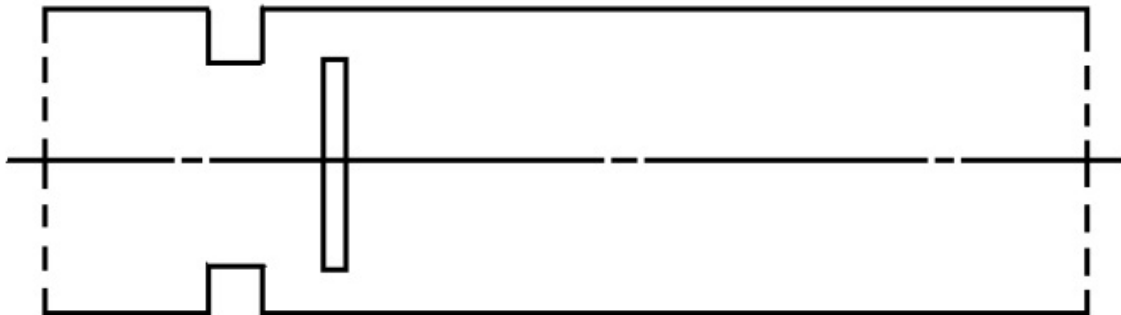
Figure 1. Flow in a channel with an obstruction (model a simplified heart valve).
