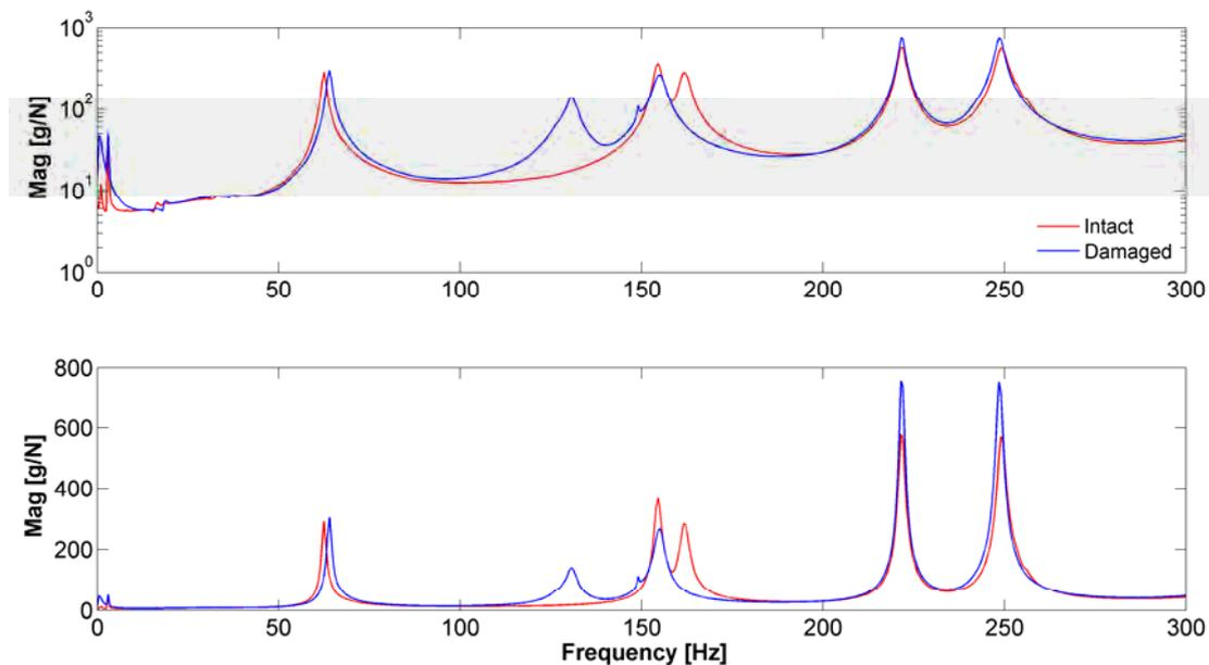
Figure 4. Experimental FRFs for intact and damaged structure - Plate 2
