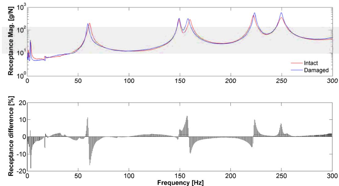
Figure 6. Experimental FRFs and the receptance differences (%) for the plate 1
