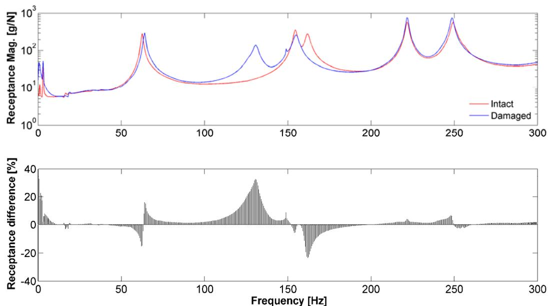
Figure 7. Experimental FRFs and the receptance differences (%) for the plate 2
