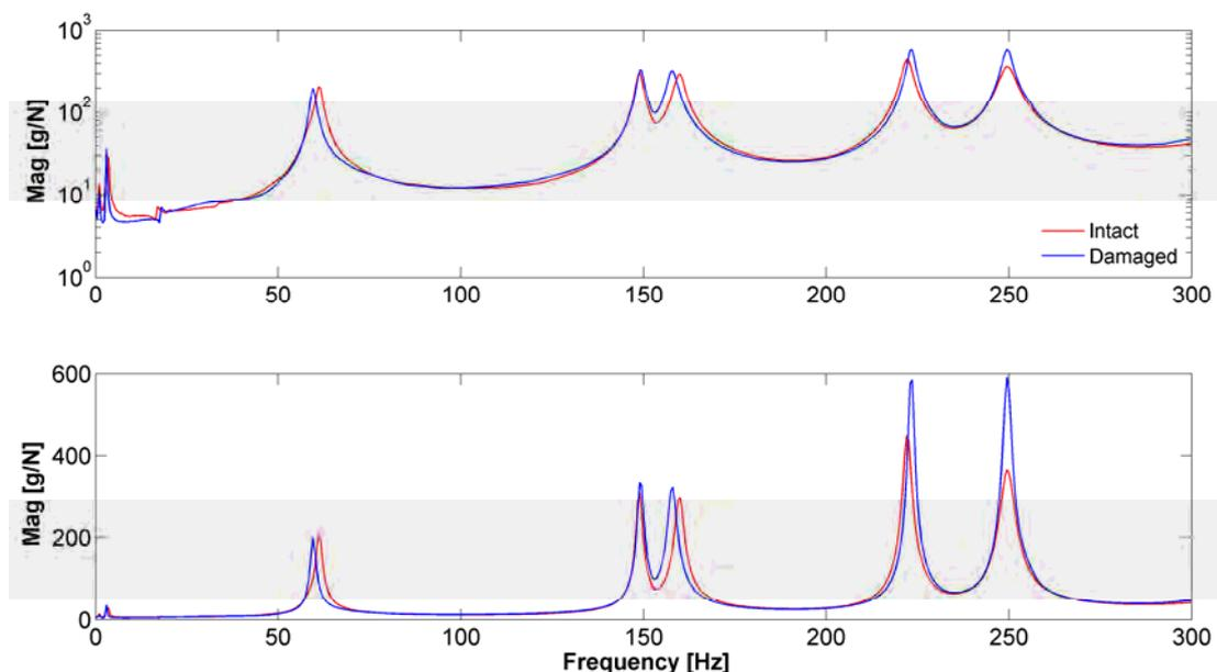
Figure 3. Experimental FRFs for intact and damaged structure - Plate 1
