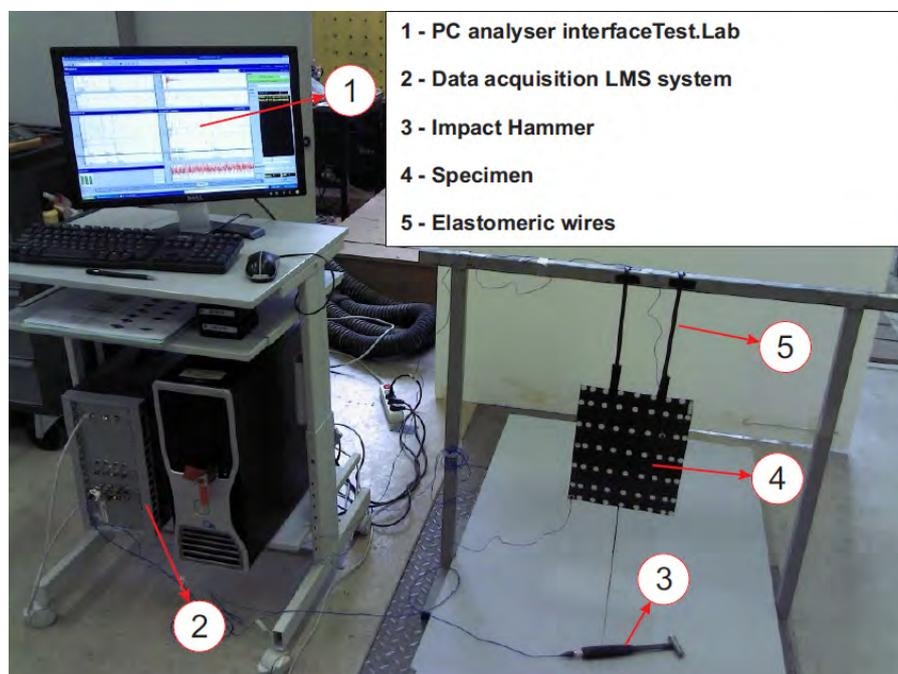
Figure 2. General layout of the used equipment
