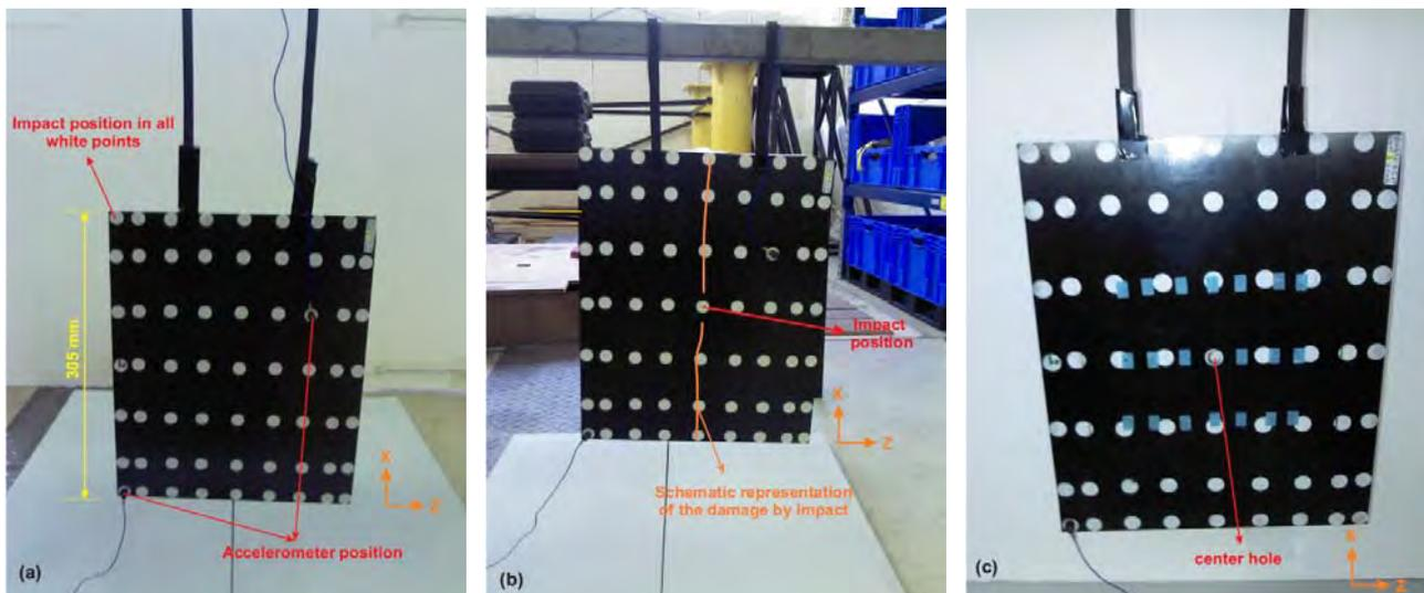
Figure 1. Experimental models: (a) Intact (b) damaged by impact and (c) damaged by a center hole
